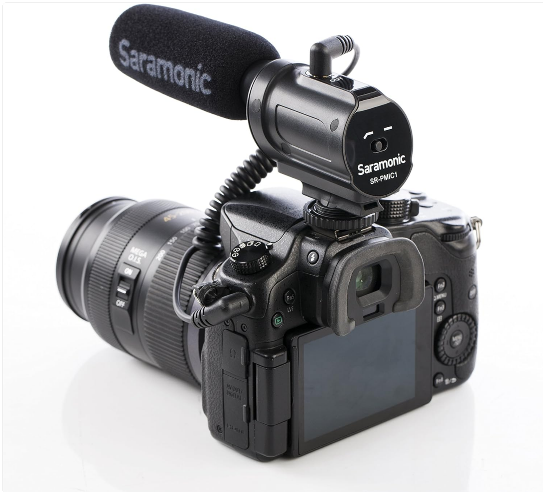
Image: The Saramonic SR-PMIC1 microphone securely mounted on a DSLR camera's hot shoe, demonstrating a typical setup configuration.
