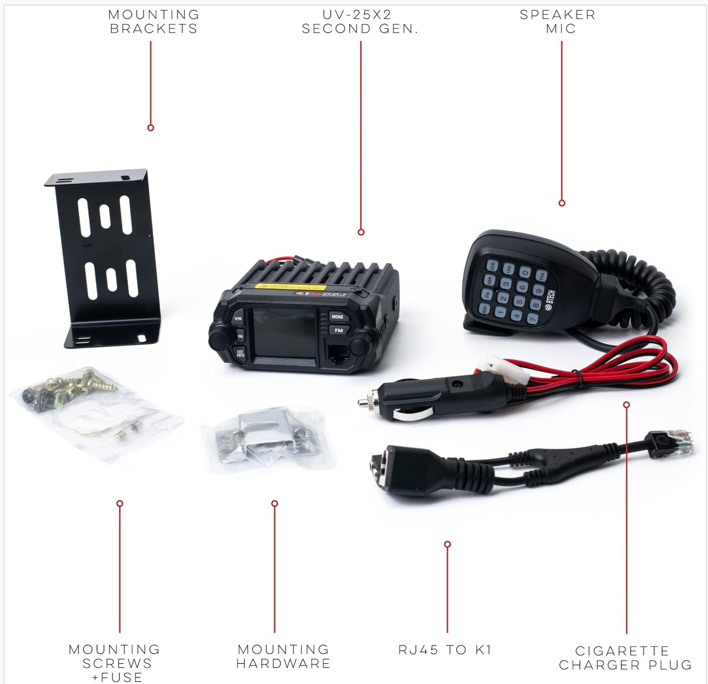
Figure 3.1: Included components of the BTECH UV-25X2 radio kit.
