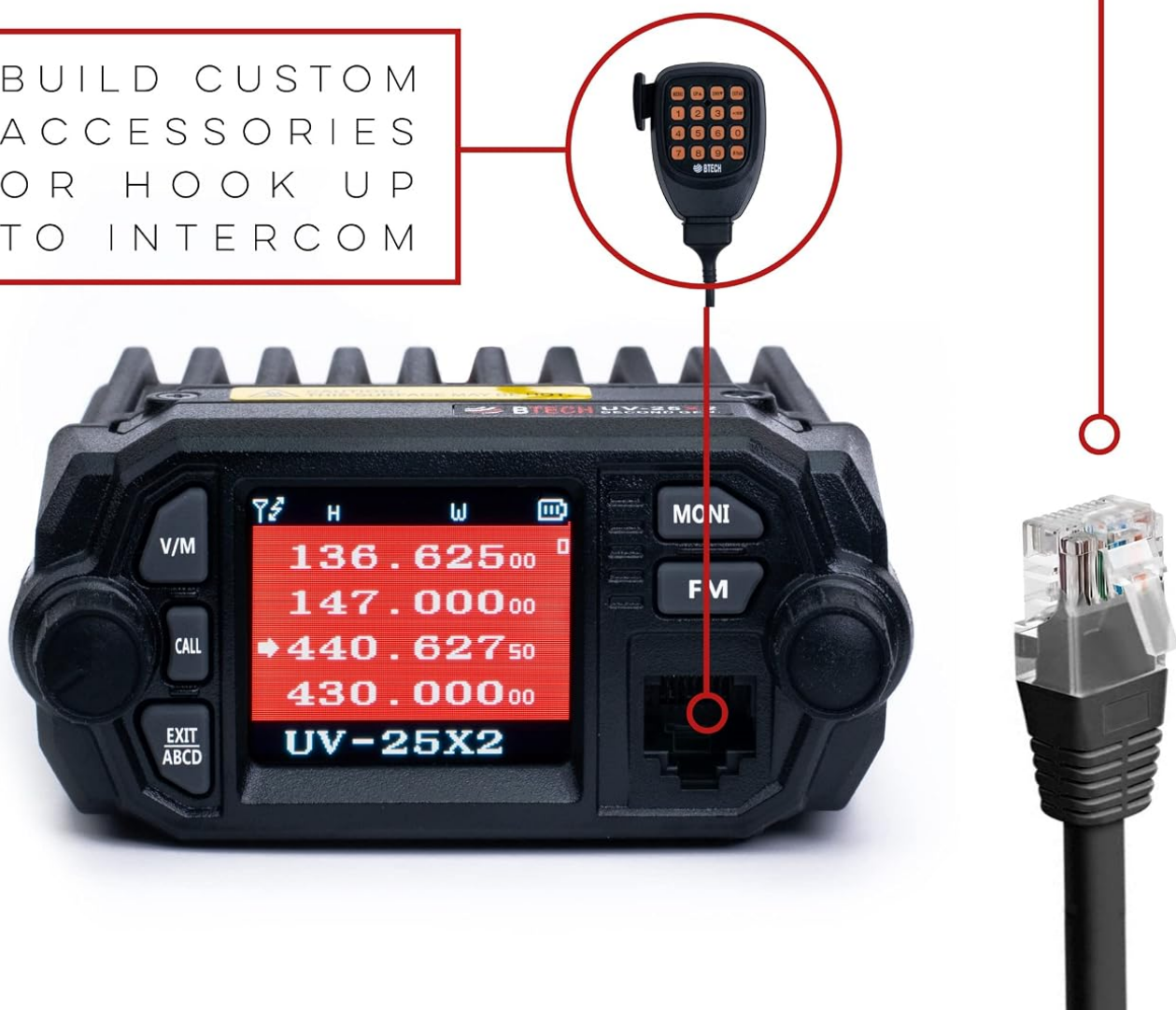
Figure 6.3: Audio I/O capabilities via the RJ45 port.
