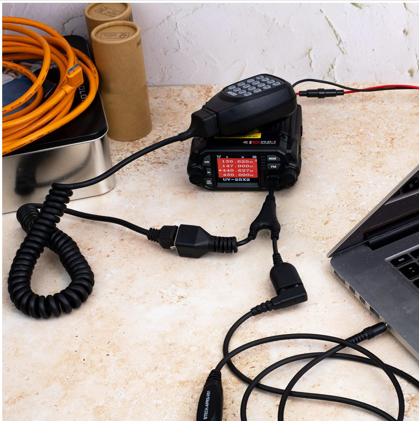
Figure 5.1: Connecting the UV-25X2 to a computer for programming.
