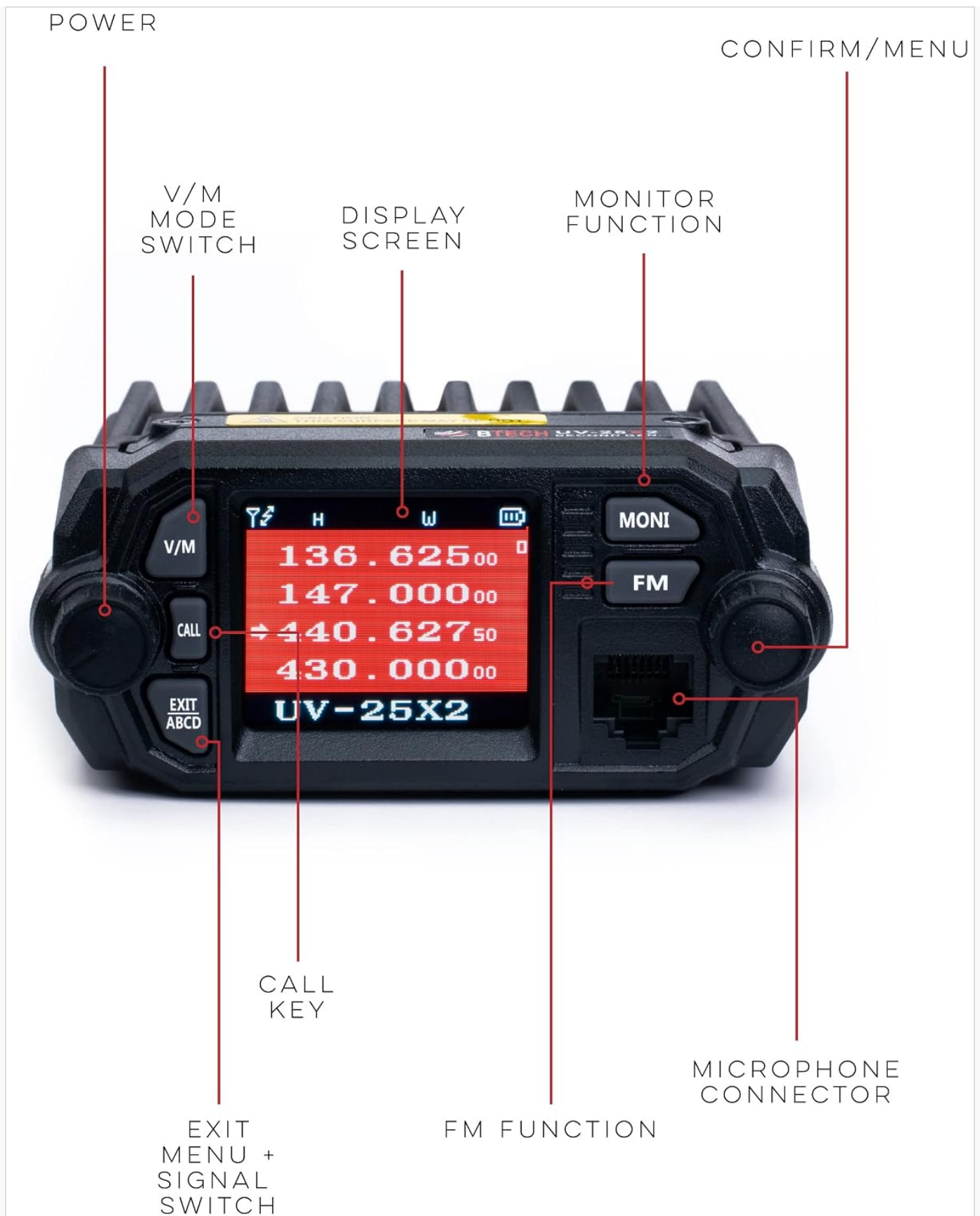
Figure 4.1: Front panel controls and connections of the UV-25X2.
