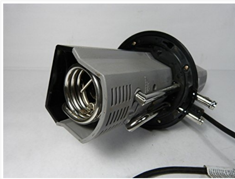
Figure 2: Underside view of the VWR 89202-918 showing the heating coil and circulation components. This image highlights the internal heating element and the pump mechanism responsible for fluid circulation within the bath.
