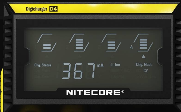
Figure 2: Close-up of the Nitecore D4's highly visible liquid crystal display, showing charging current and other parameters.
