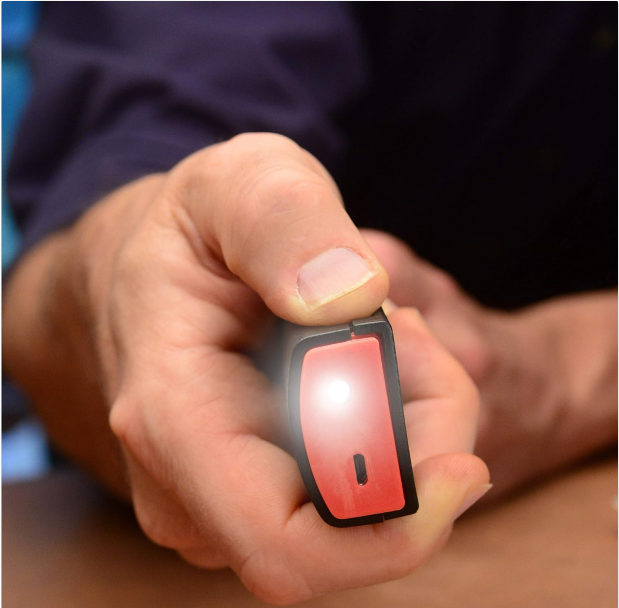
Figure 4: The DMXcat's integrated flashlight in operation, providing illumination for working in low-light conditions.
