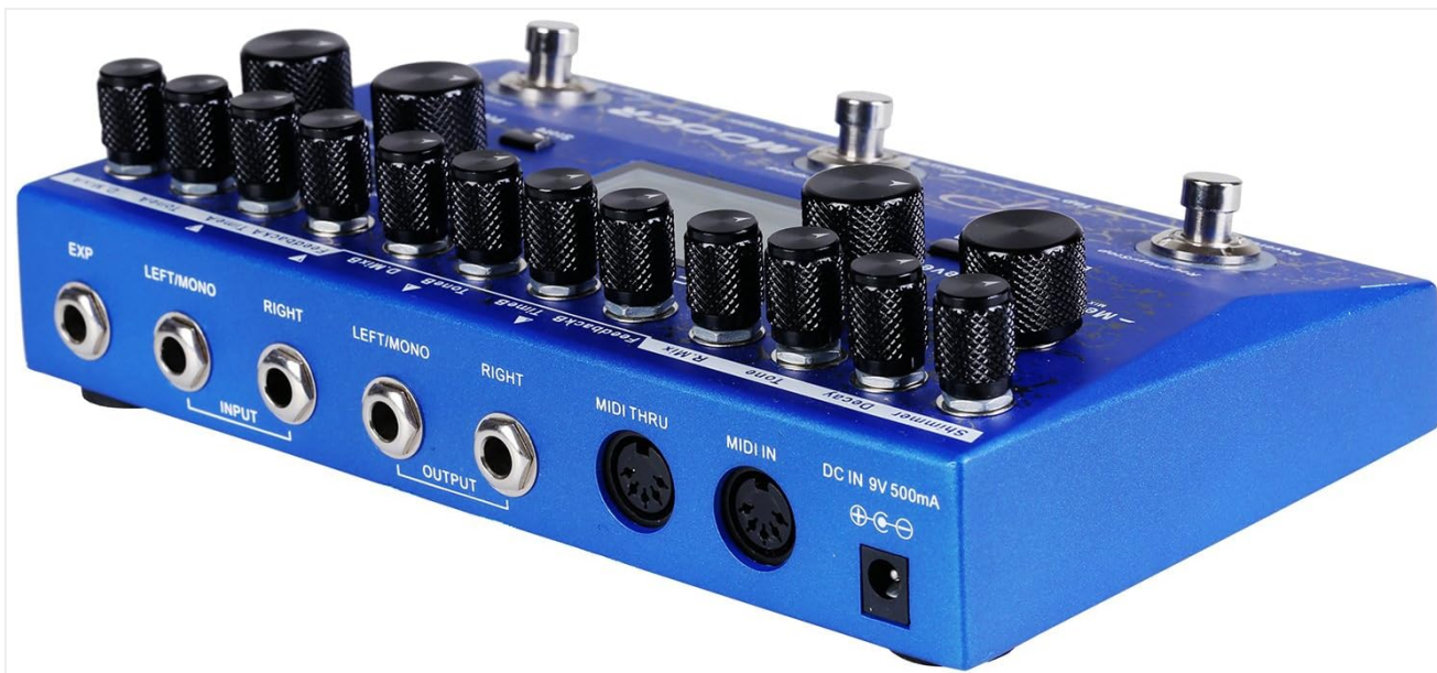
Figure 2: Rear view of the MOOER Ocean Machine TDL3, showing input/output jacks, MIDI ports, and power input.
