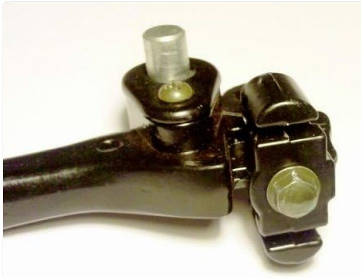
Figure 3: Close-up view of the brake lever's mounting point and pivot. This image details the bolt and pin mechanism used for securing the lever and its pivot action.
