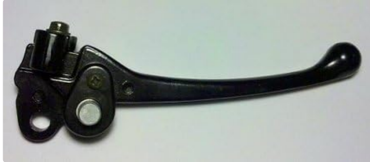
Figure 2: Side view of the Right Brake Lever Handle. This perspective highlights the lever's ergonomic curve and the mounting points for attachment to the handlebar.
