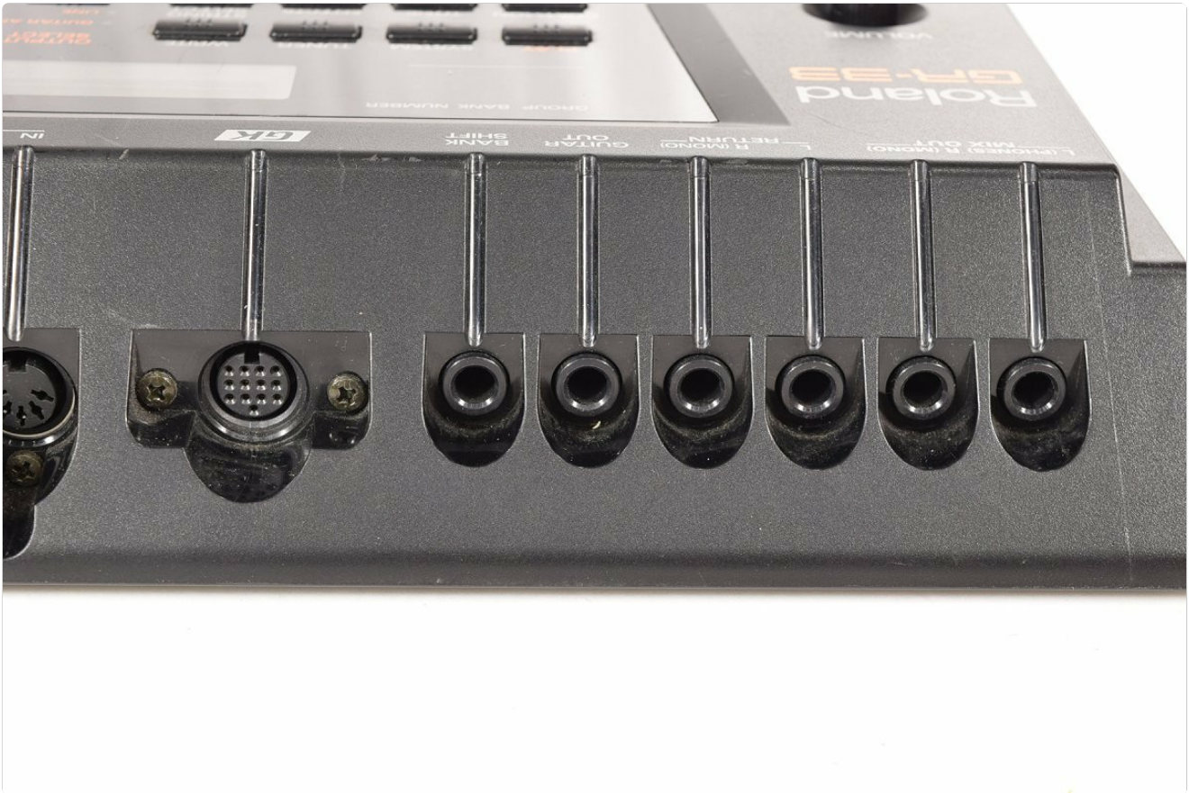
Figure 4.3: Detailed view of the GK IN, GUITAR OUT, GUITAR RETURN, and L/R MIX OUT jacks on the GR-33 rear panel.
