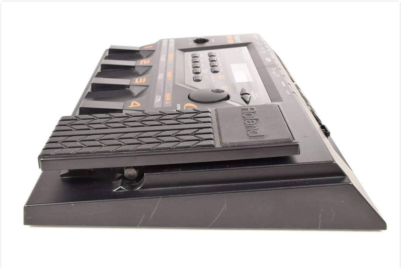
Figure 5.2: Side view of the GR-33, highlighting the expression pedal for real-time control of effects and parameters.
