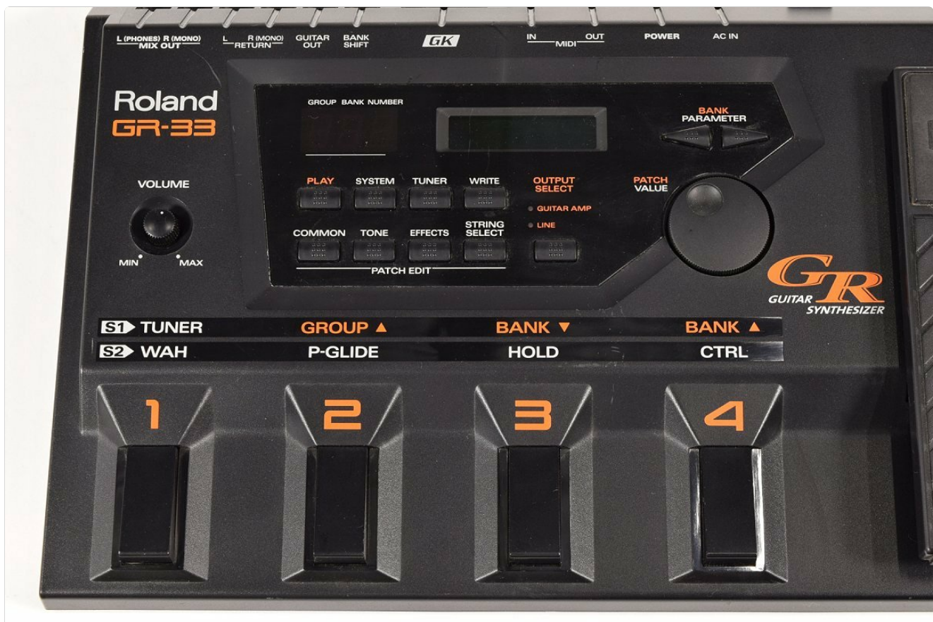
Figure 5.1: Close-up view of the GR-33's main control panel, including the display, navigation buttons, and patch edit controls.
