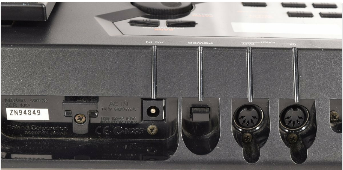
Figure 4.1: Rear panel of the GR-33, showing the AC IN, MIDI IN/OUT, GK IN, GUITAR OUT, GUITAR RETURN, and L/R MIX OUT jacks.
