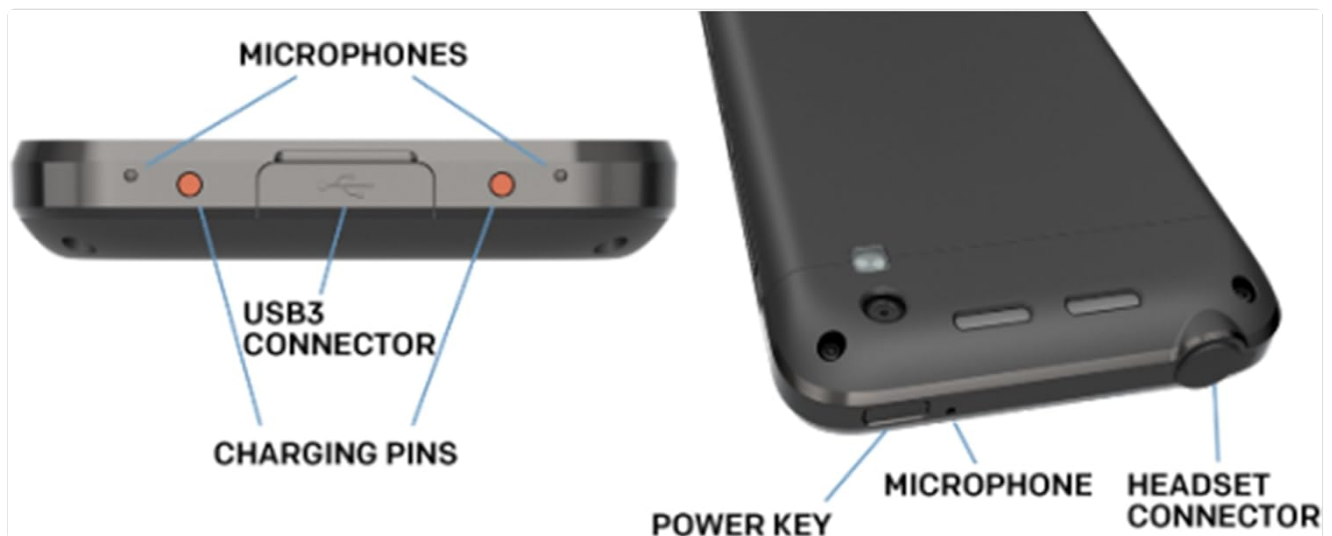
Figure 3.4: Top and bottom views of the Bittium Tough Mobile, indicating the locations of microphones, the USB3 connector, charging pins, the power key, and the headset connector.
