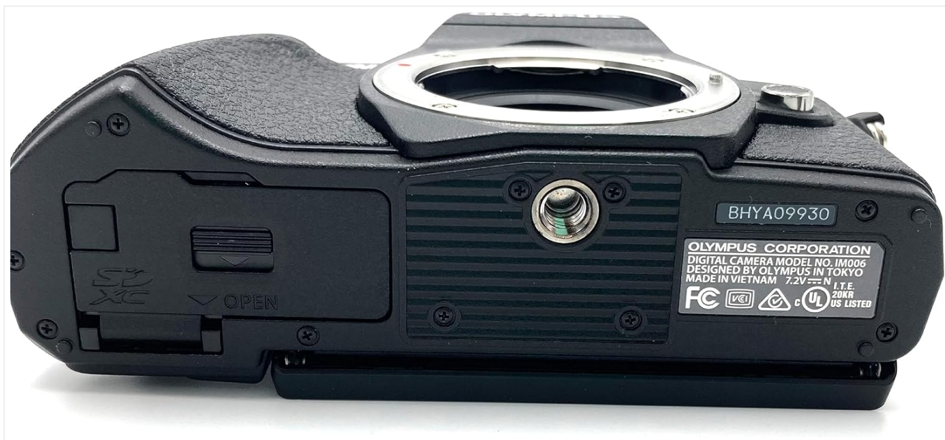
Image: The bottom of the camera, illustrating the battery and SD card compartment.
