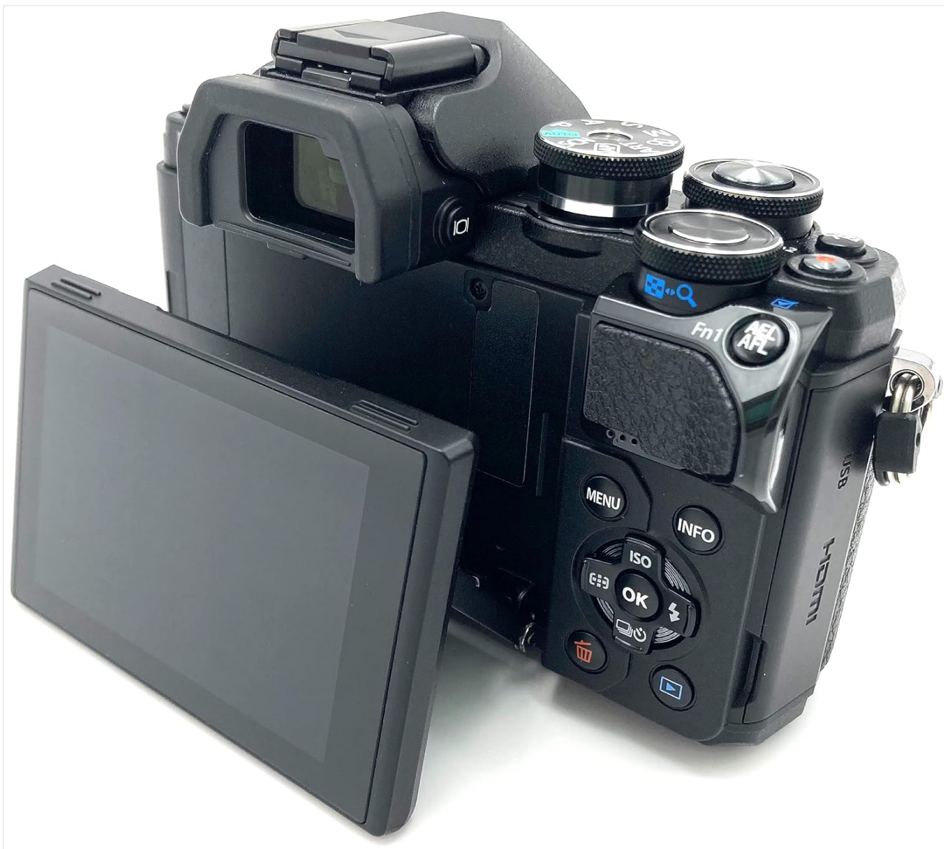
Image: Rear view of the camera with the articulated LCD screen tilted for flexible viewing angles.
