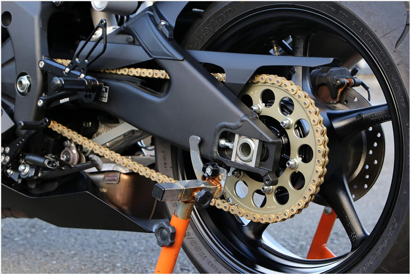
Figure 2: The SUNSTAR rear sprocket correctly installed on a motorcycle, demonstrating proper fitment and alignment with the chain.
