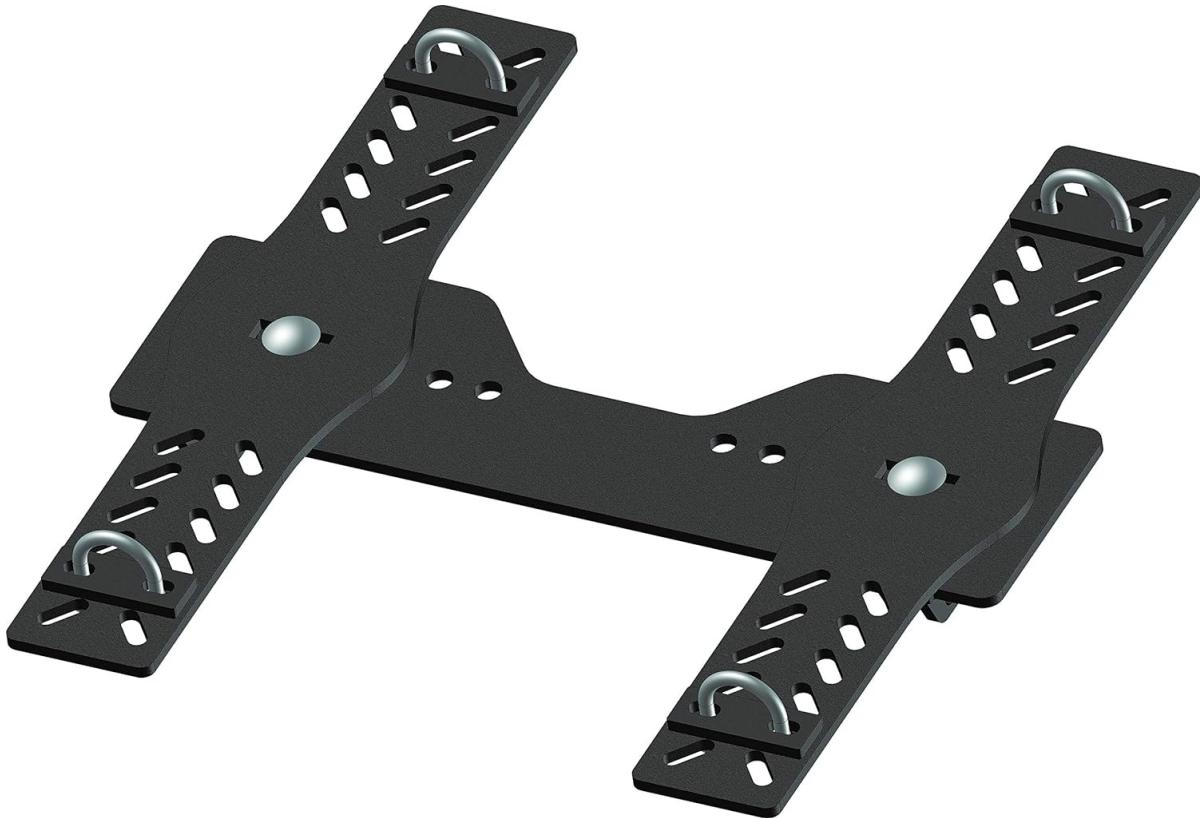
An illustration of the KFI Products 105745 Universal ATV Plow Mount, showing its three main components and attachment points. The mount is black, made of Grade 50 steel with a powder-coated finish, and features multiple adjustment slots and four U-bolt attachment points for securing to an ATV frame.
