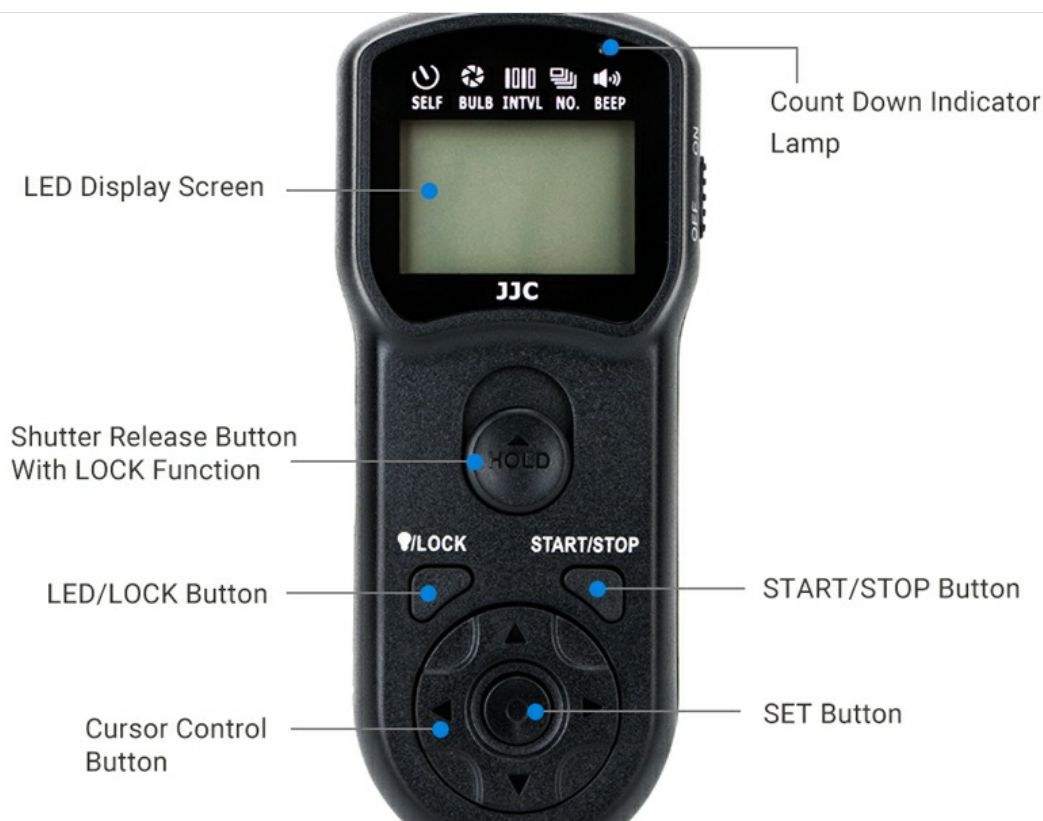
Figure 4: Overview of the intervalometer's controls, including the LED display screen, shutter release button with lock function, LED/LOCK button, START/STOP button, SET button, and cursor control buttons.
