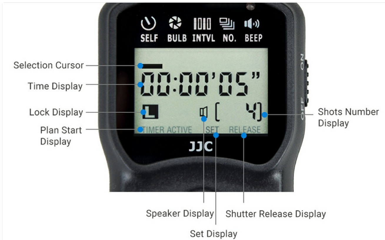
Figure 5: Detailed view of the LCD screen indicating selection cursor, time display, lock display, plan start display, speaker display, set display, and shots number display.
