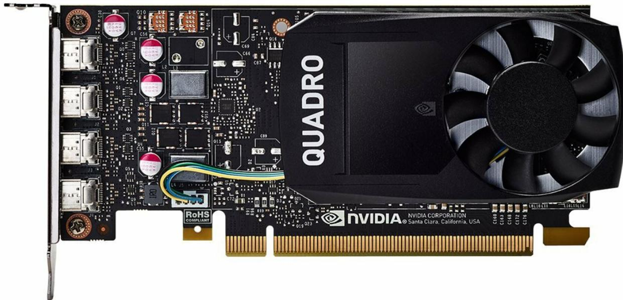
Image: The PNY NVIDIA Quadro P1000 Professional Graphics Board, a compact graphics card with a single fan and multiple display outputs.
