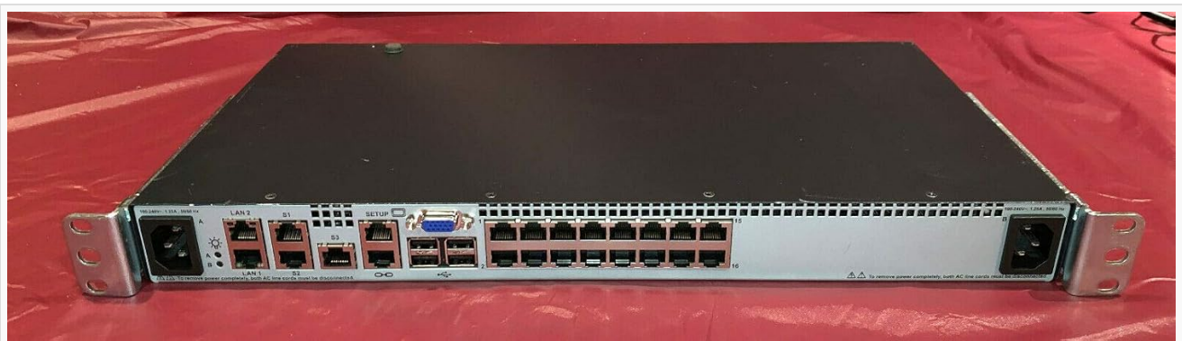
Figure 2: Rear panel of the HP AF621A Digital KVM Switch. This image highlights the various connectivity options, including dual power inputs, two LAN ports (LAN 1, LAN 2), a VGA setup port, USB ports for local console peripherals, and 16 dedicated KVM ports for connecting managed servers. Also visible are the tiering port and a serial port.
