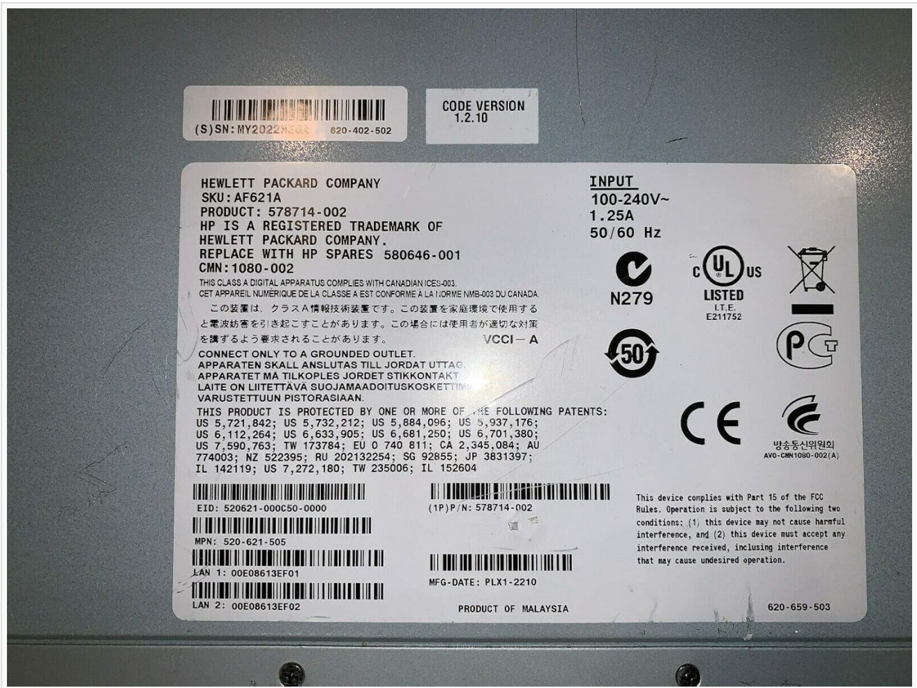
Figure 3: Product label details for the HP AF621A KVM Switch. This label provides critical information such as the SKU, input power requirements (100-240V~, 1.25A, 50/60 Hz), various regulatory compliance marks (UL, CE, VCCI, N279), and specific manufacturing and serial numbers like SKU: AF621A, Product: 578714-002, CPN: 1080-002, and LAN MAC addresses.
