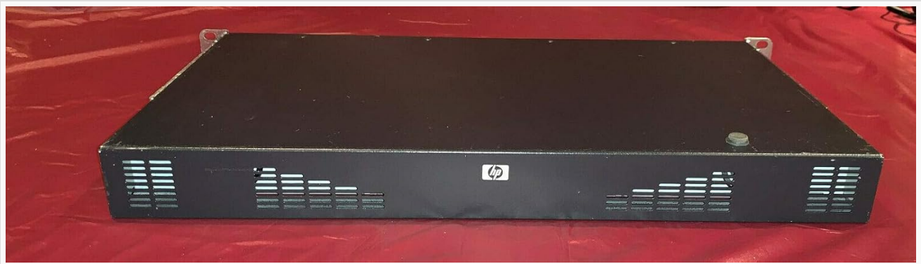
Figure 1: Front view of the HP AF621A Digital KVM Switch. This view shows the compact 1U rack-mountable design with the HP logo centrally placed and ventilation grilles on either side, ensuring proper airflow for internal components.
