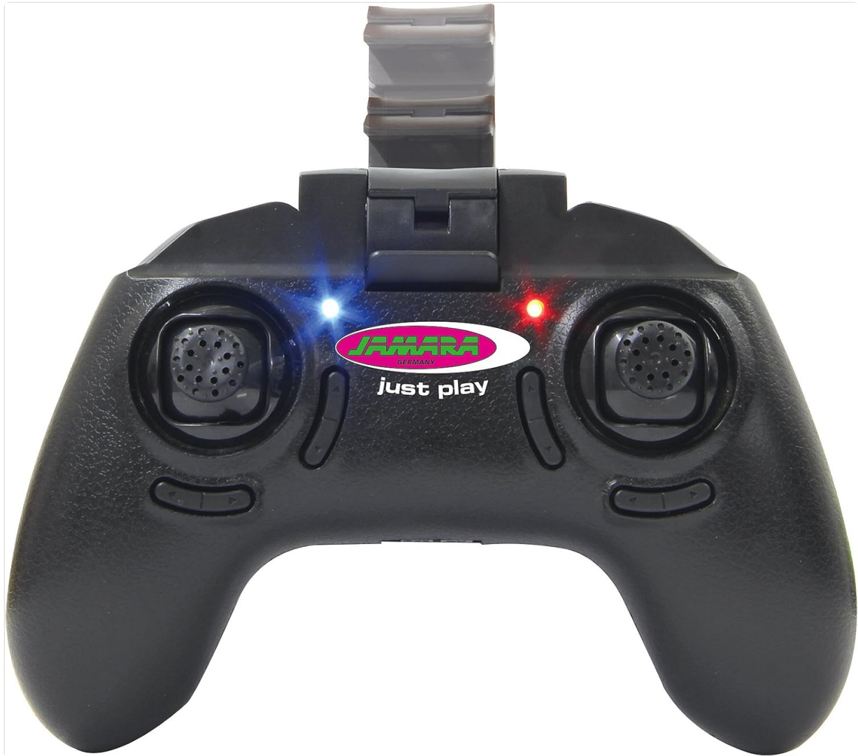
Image 4.2: The 2.4 GHz remote control for the quadrocopter.
