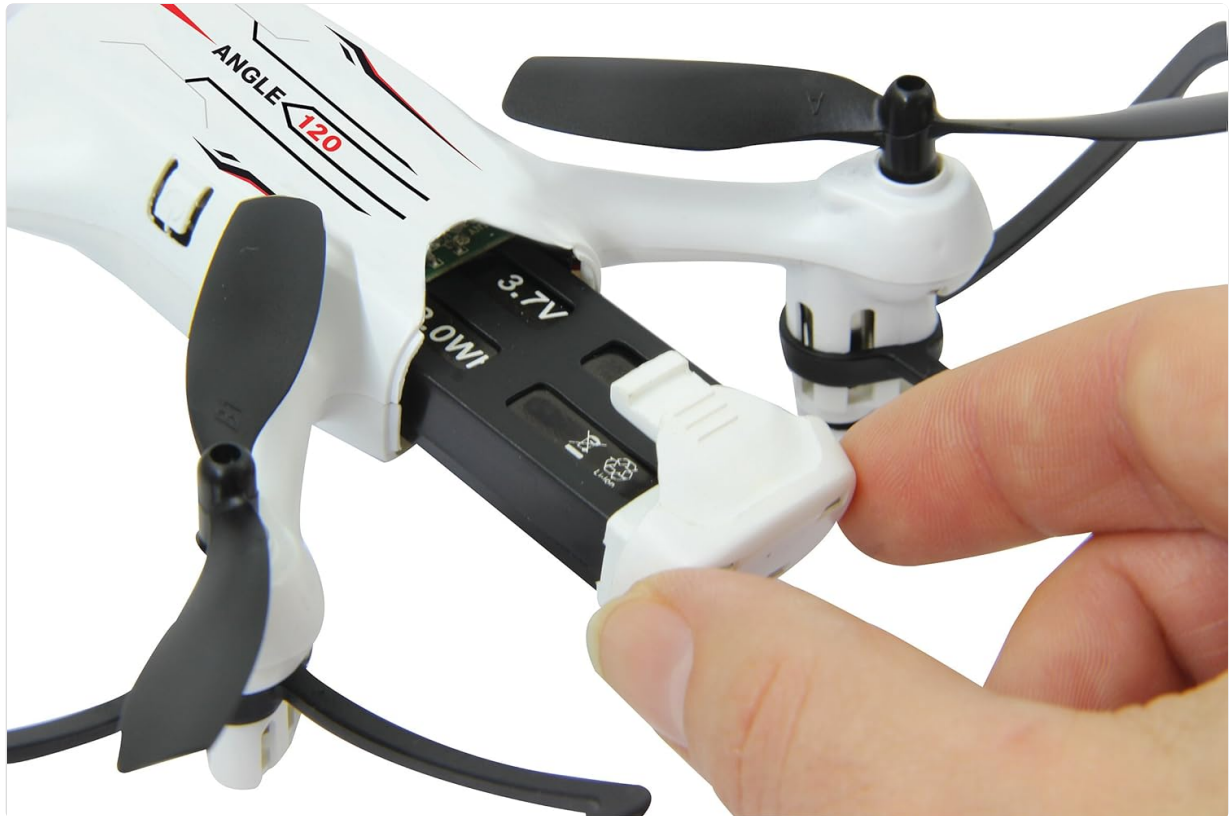
Image 4.1: Inserting the rechargeable battery into the quadrocopter.
