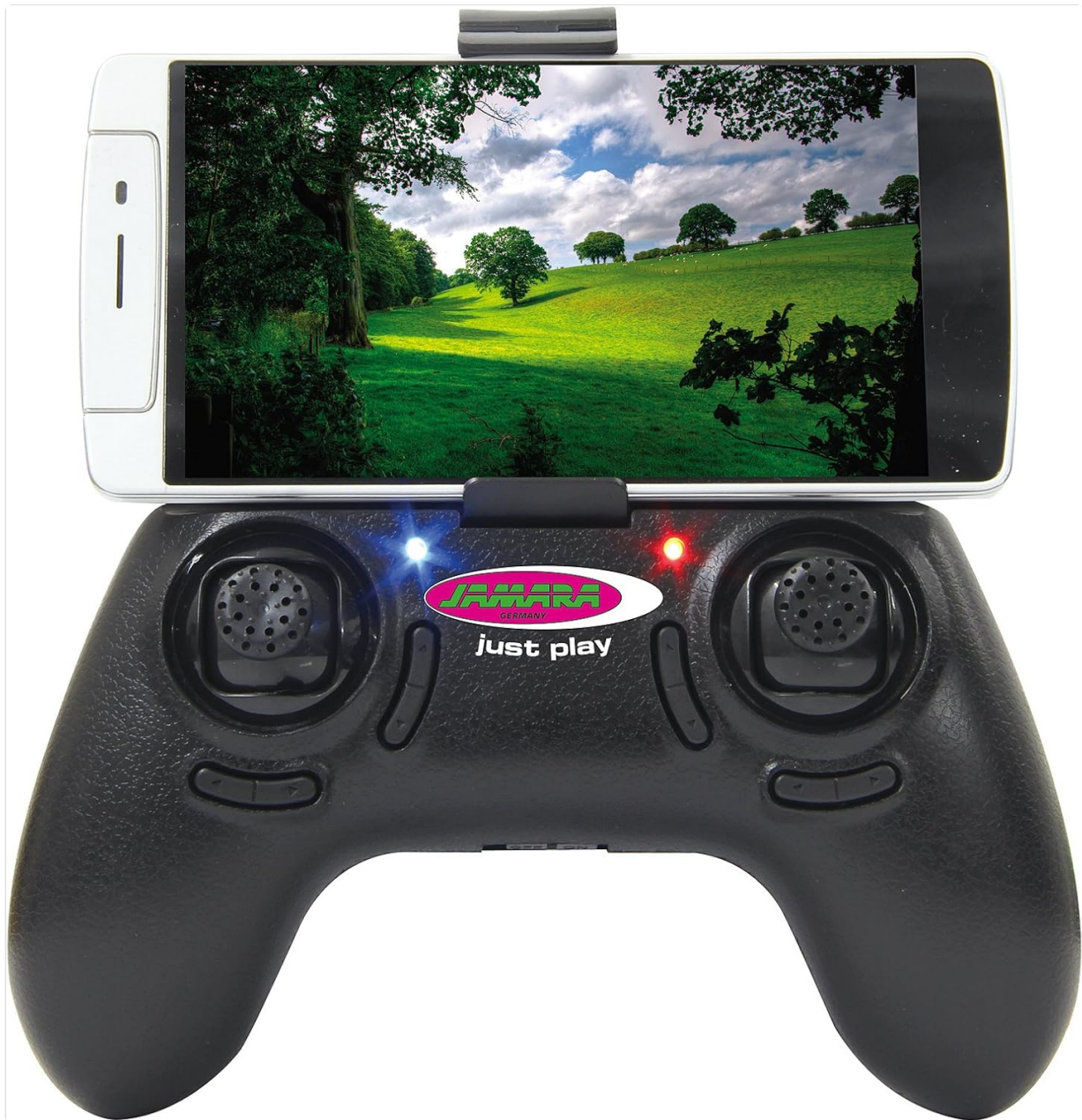
Image 4.4: Remote control with a smartphone attached for FPV viewing.
