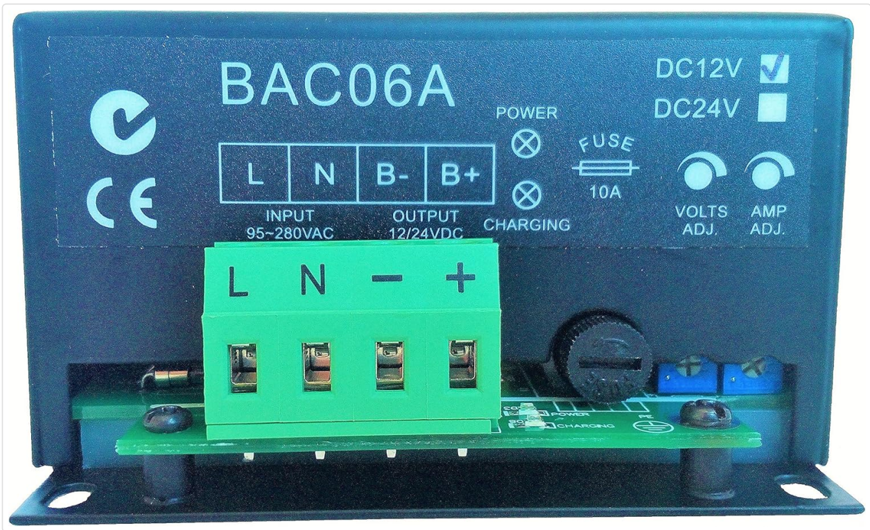
Figure 2: Close-up of the terminal block, showing 'L' and 'N' for AC input, and '-' and '+' for DC output. Also visible are the 'VOLTS ADJ.' and 'AMP ADJ.' potentiometers and LED indicators.
