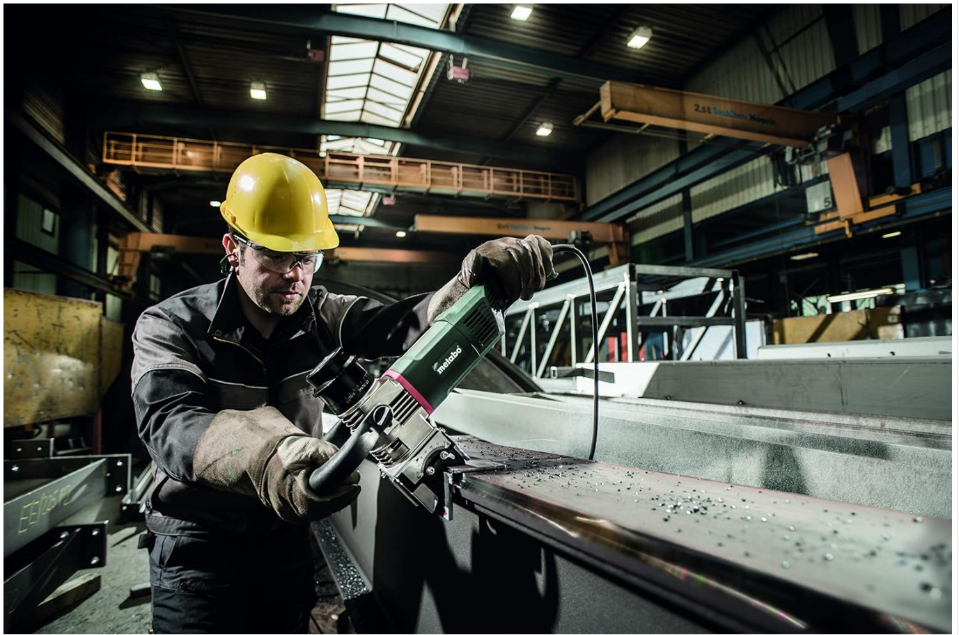
Figure 4: Beveling a metal beam with the Metabo tool.
