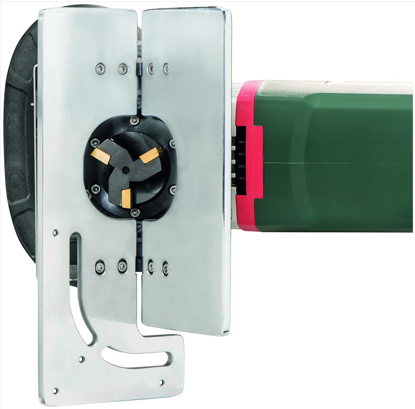
Figure 6: Inspecting the universal carbide burr with three carbide inserts.
