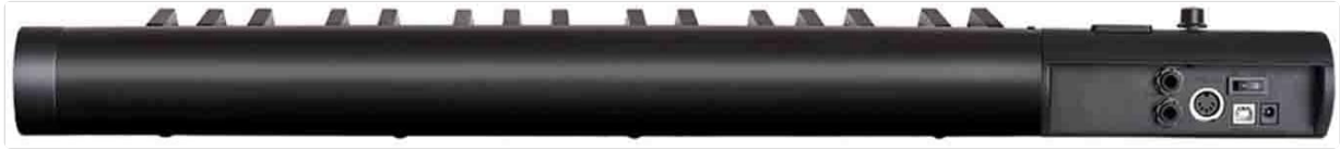
Image 4.1: Rear panel of the ICON iKeyboard 4X, illustrating the USB, MIDI OUT, and DC IN ports for connectivity.
