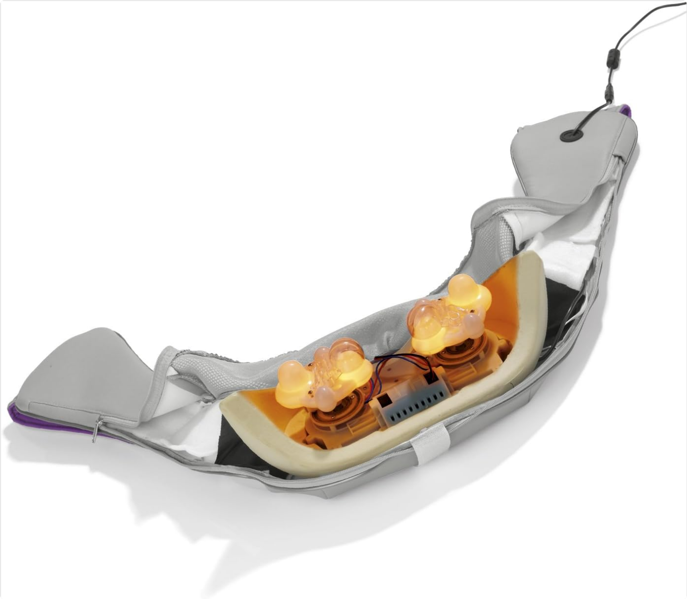
Figure 5: Internal view of the massager, illustrating the rotating massage nodes.
