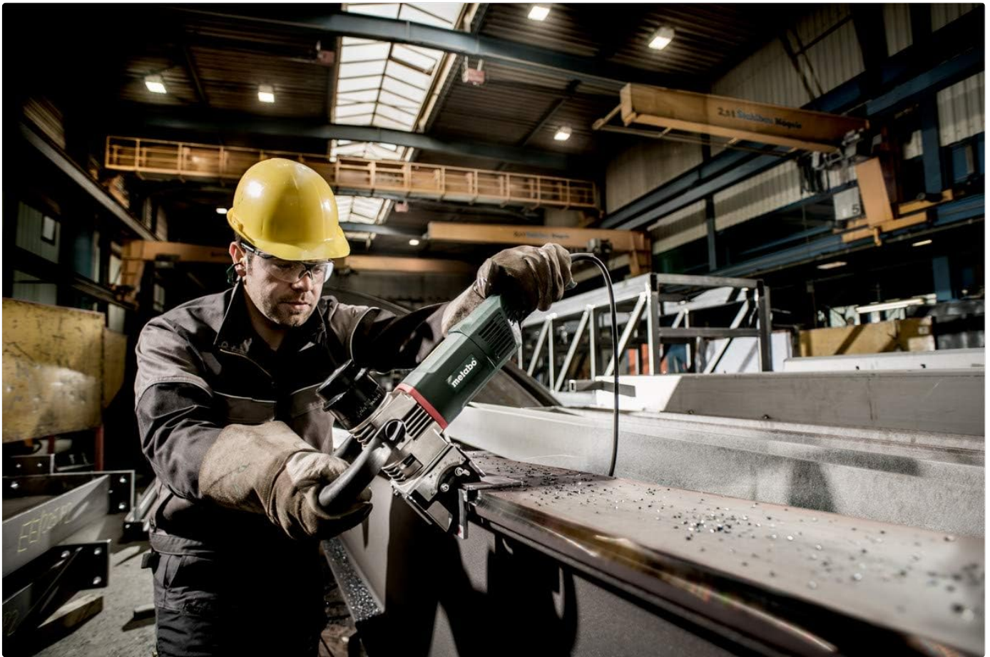
Figure 6: The tool in operation, demonstrating its use on a flat metal edge for weld preparation.
