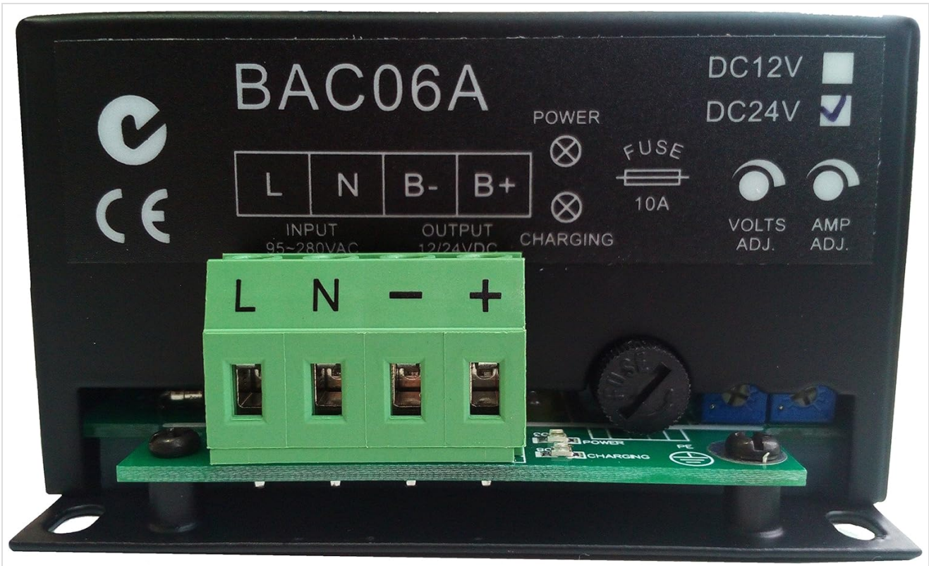
Figure 3.1: Front view of the BAC06A-24V charger. This image displays the input terminals (L, N), output terminals (B-, B+), fuse, LED indicators for Power and Charging, and adjustment potentiometers for voltage and current.
