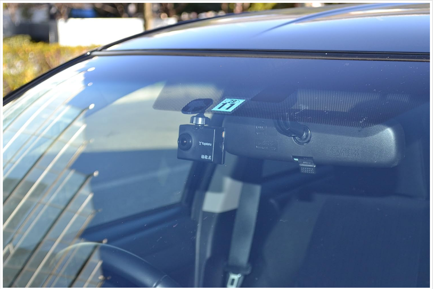
Image: The dash camera mounted on the inside of a car windshield, positioned to record the road.
