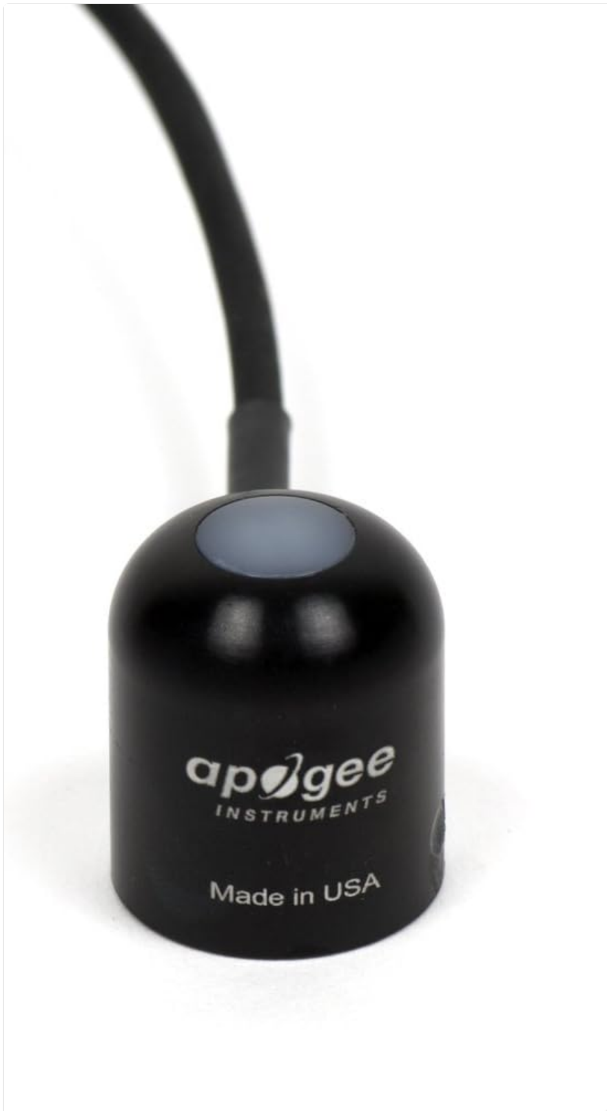
Figure 2: Close-up view of the Apogee waterproof quantum sensor. This image highlights the robust, anodized aluminum body and the acrylic diffuser of the sensor head. The sensor contains a blue-enhanced silicon photodiode and custom optical filters, designed for accurate underwater PAR measurements.
