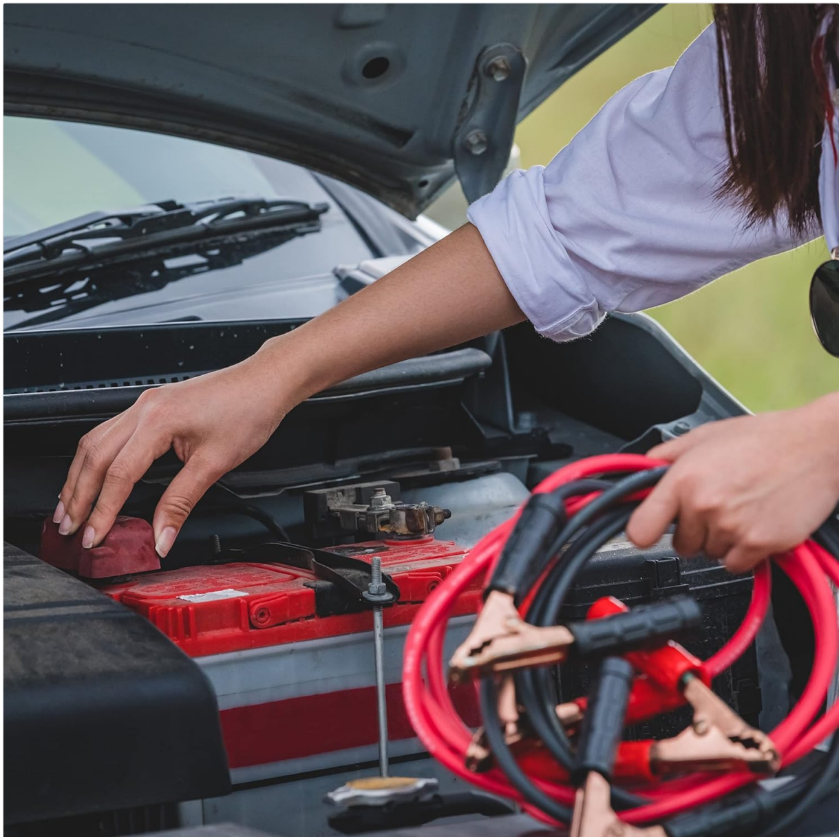
Figure 5: Demonstrating the connection of jumper cables to a car battery, a crucial step in jump-starting a vehicle.
