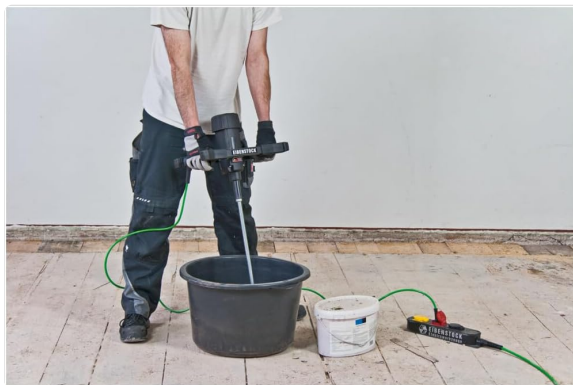
Image 4: The mixer in operation, showing the power cord connected and the paddle submerged in a large mixing tub.
