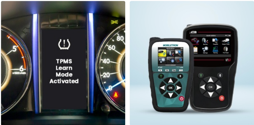
Figure 4: TPMS Learn Mode and Compatible Relearn Tools
