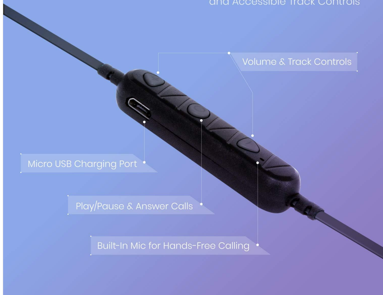
Figure 2.1: Close-up of the inline remote showing the Micro USB charging port.
