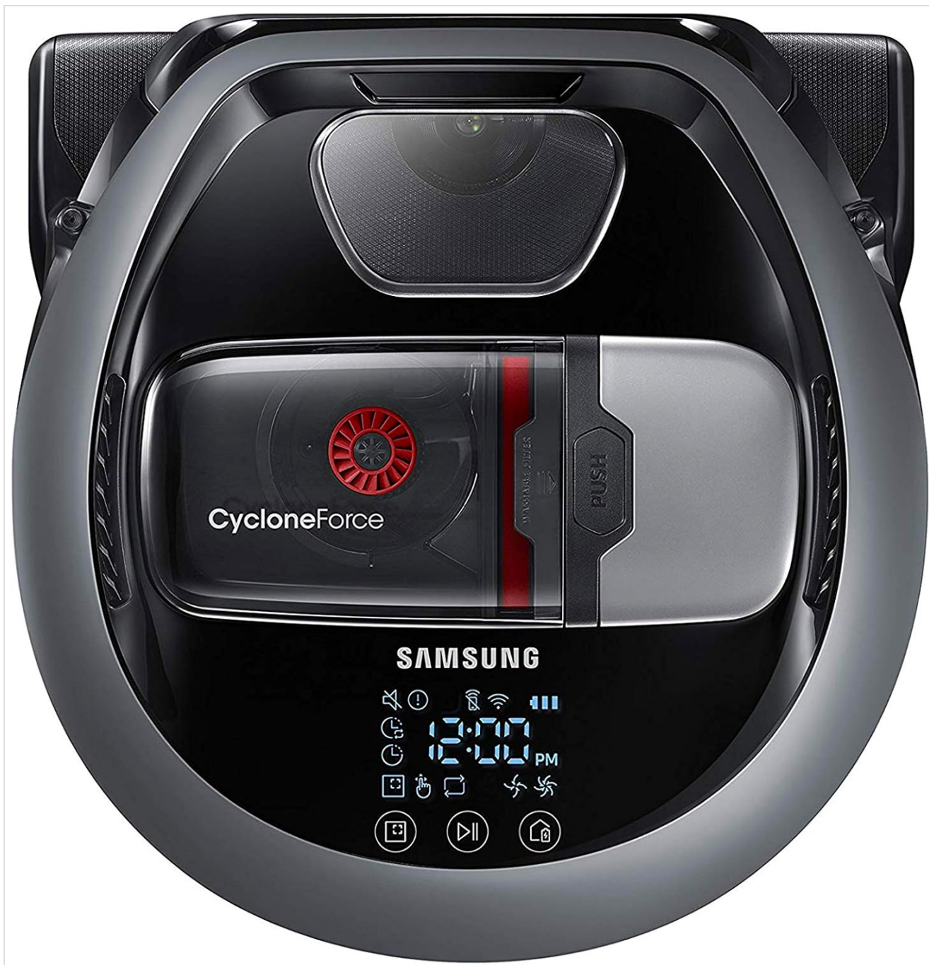
Image: A top-down view of the Samsung POWERbot R7040, highlighting the CycloneForce dustbin.
