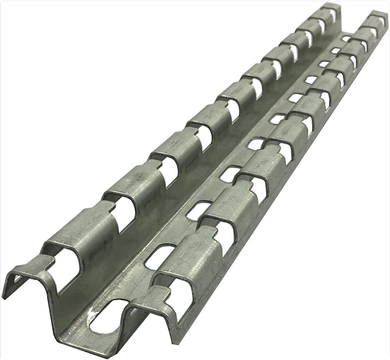
Figure 1: The Legrand-Cablofil FASP400PG Mounting Bracket. This image displays the Legrand-Cablofil FASP400PG Mounting Bracket. It is a long, metallic profile designed with a series of interlocking tabs and slots along its length, facilitating the secure attachment of Cablofil wire mesh trays without the need for additional nuts and bolts. The bracket features a U-shaped cross-section, providing structural integrity for mounting applications.
