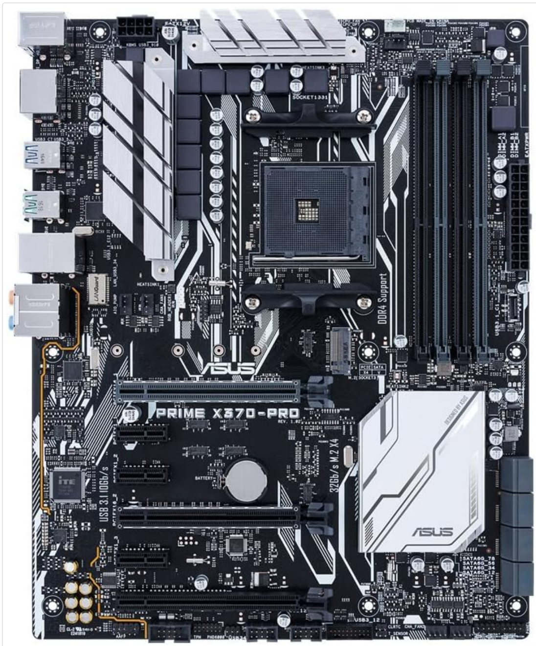
Figure 2.1: ASUS Prime X370-Pro Motherboard. This image displays the full layout of the motherboard, highlighting the CPU socket, RAM slots, PCIe slots, M.2 slot, and various headers and ports.
