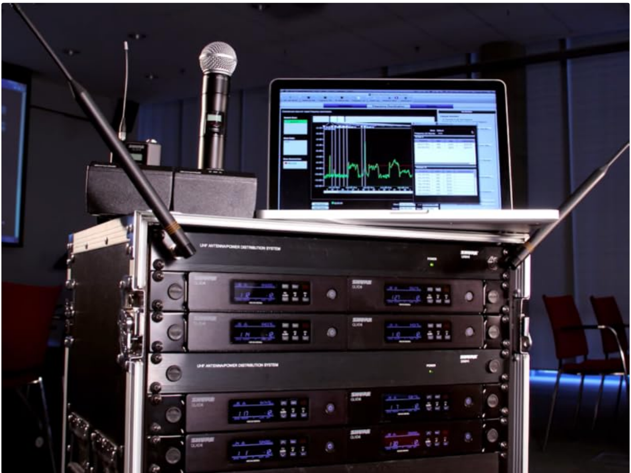
Image: Multiple Shure QLX-D wireless receivers in a rack, connected to a laptop for network scanning.
