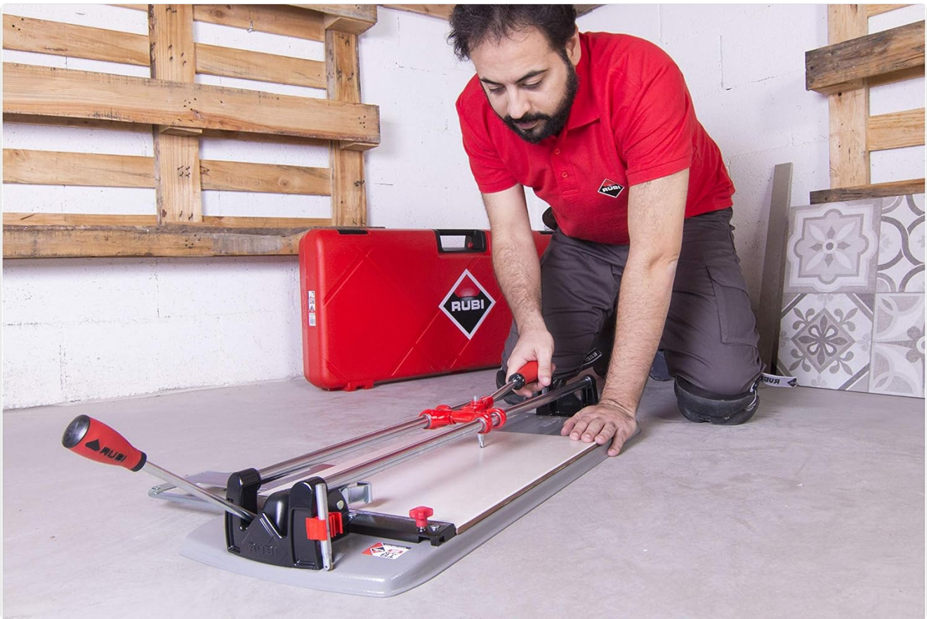
Image: A user demonstrating the scoring process on a tile using the RUBI TS-43 MAX manual tile cutter.
