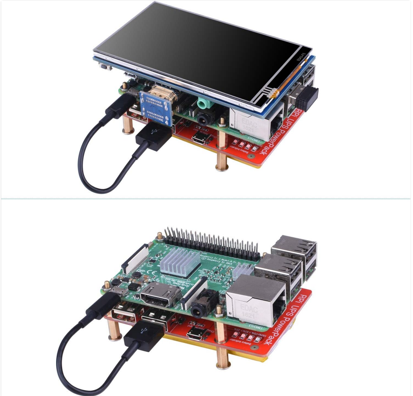
Figure 5.1: Example of the UPS Battery Pack connected to a Raspberry Pi with a display.
