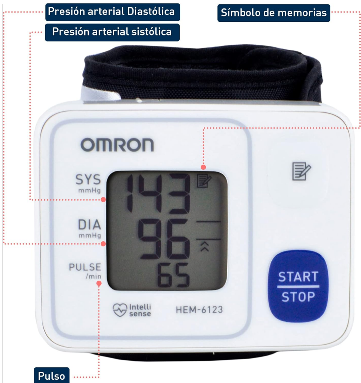
Image 3.2: Display Indicators. This image highlights the different sections of the monitor's display, indicating where systolic pressure, diastolic pressure, pulse rate, and the memory symbol are shown.
