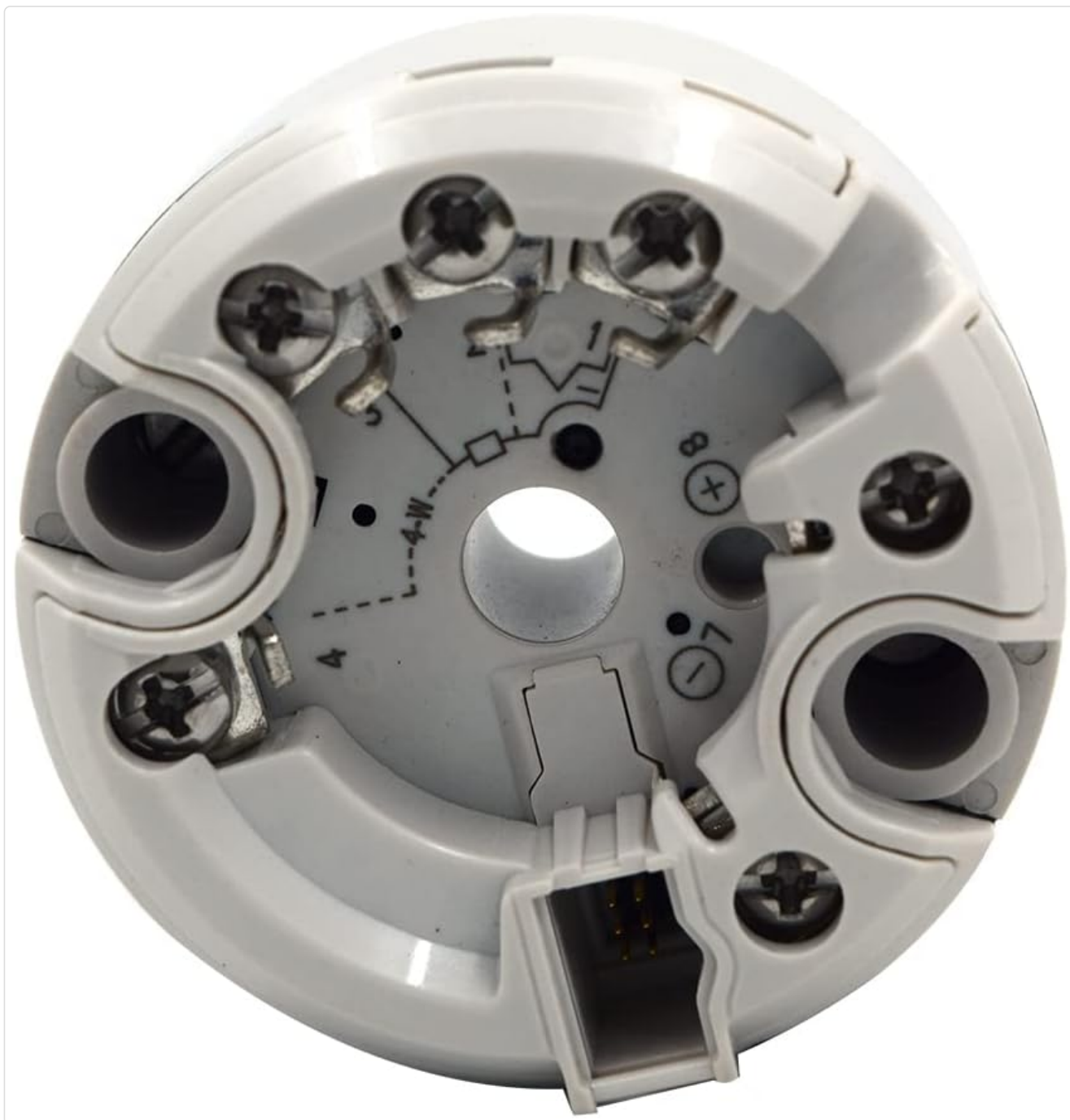
Figure 4.2: Another internal view of the ABB TTH200 Temperature Transmitter, highlighting the terminal screws and the central opening for sensor wiring. This perspective shows the depth of the terminal block.
