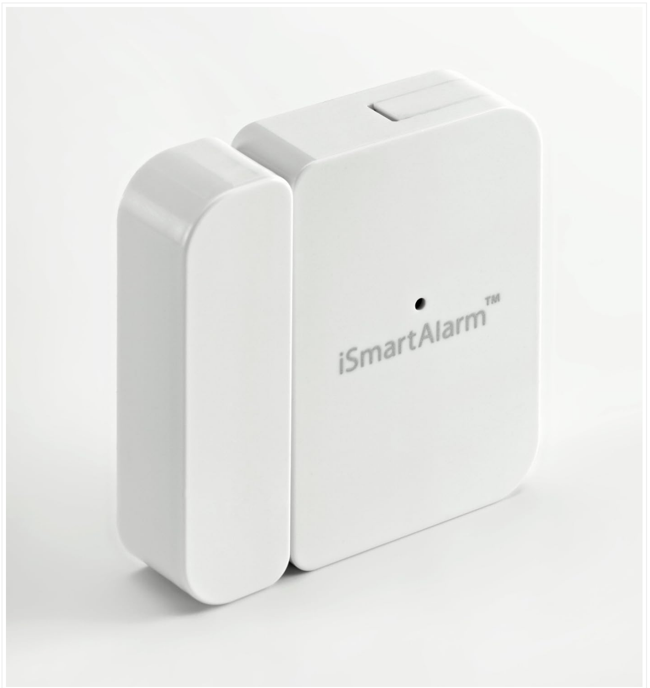
Figure 4: An iSmartAlarm Contact Sensor, used for doors and windows.
