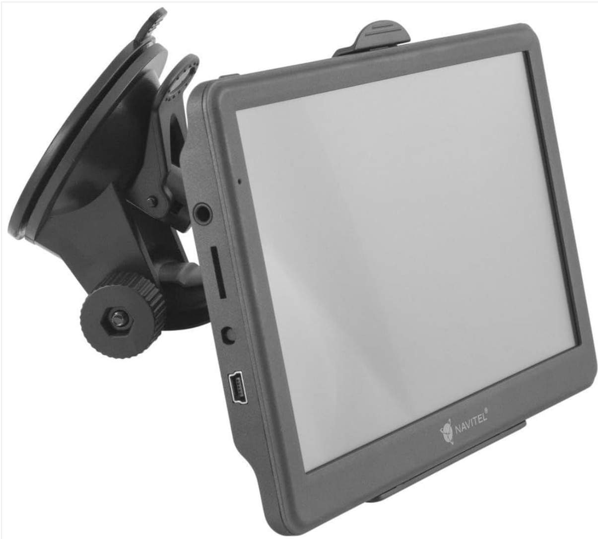
Image: The Navitel E700 navigation device with the suction cup mount attached, showing the side ports including the mini-USB and SD card slot.
