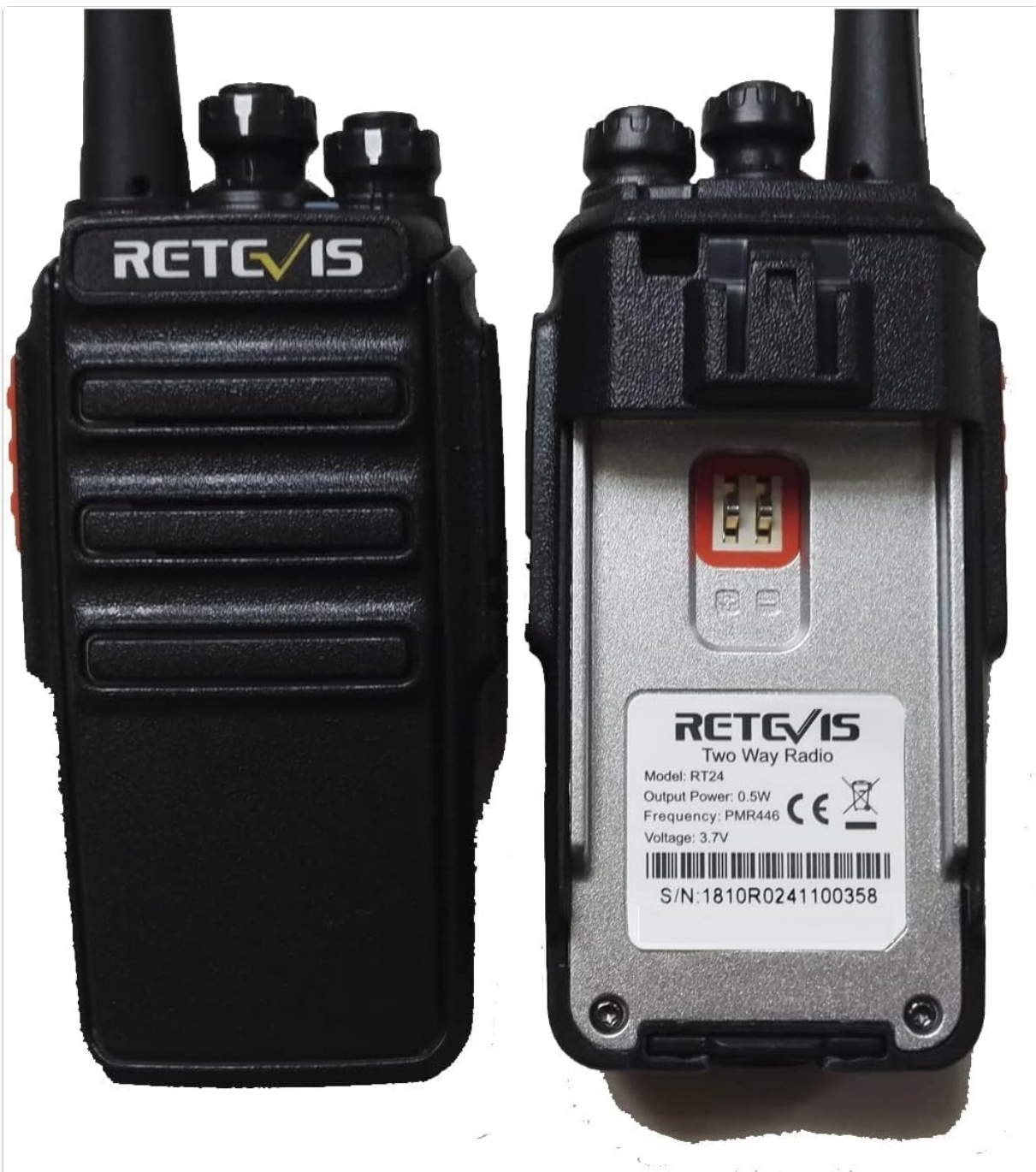
Figure 8: The rear view of the walkie talkie, displaying the model number (RT24), output power (0.5W), frequency (PMR446), voltage (3.7V), and regulatory marks (CE, RoHS).
