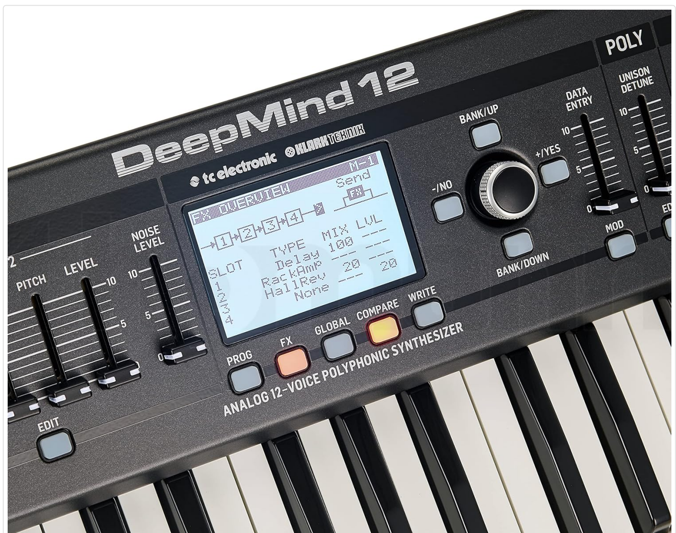
Figure 4.2: Close-up of the DeepMind 12 display and navigation controls, used for selecting presets and adjusting parameters.
