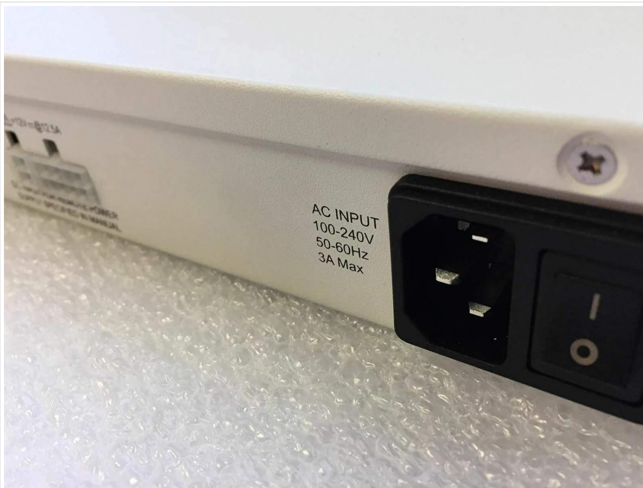
Image 2.2.1: Rear panel with AC input (100-240V, 50-60Hz, 3A Max) and power switch. Ensure the power switch is in the OFF position before connecting the power cable.
