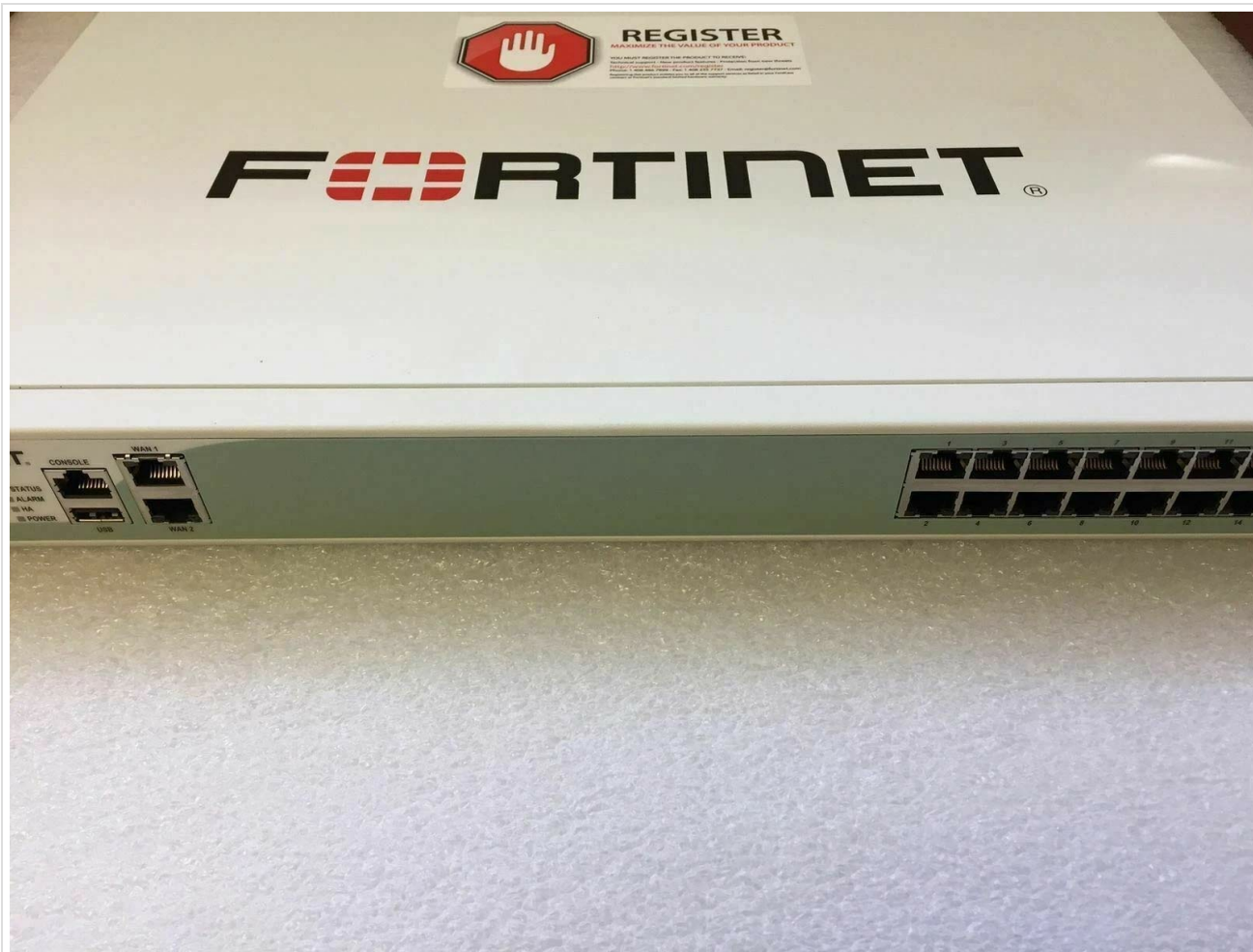
Image 2.3.1: Front panel of the FortiGate-200D, displaying the USB MGMT, MGMT, CONSOLE, STATUS, HA, ALARM, and POWER indicators, along with various RJ45 and SFP ports for network connectivity.
