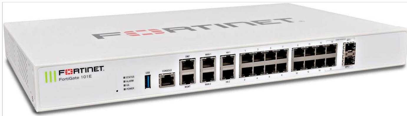
Figure 4.1: Front view of the FortiGate-101E appliance, showing the status LEDs, USB port, Console port, and various Ethernet and SFP ports for network connectivity.
