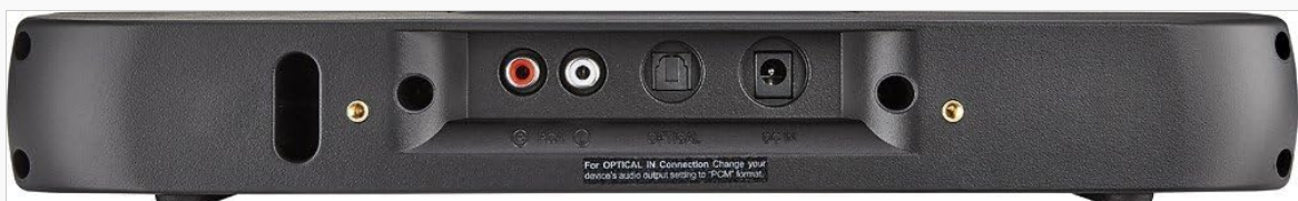
Image 4.3: Rear view of the Insignia NS-SB216 Mini Soundbar. This image displays the various input ports including RCA (red and white), Optical, and the DC power input, along with wall-mount screw holes.
