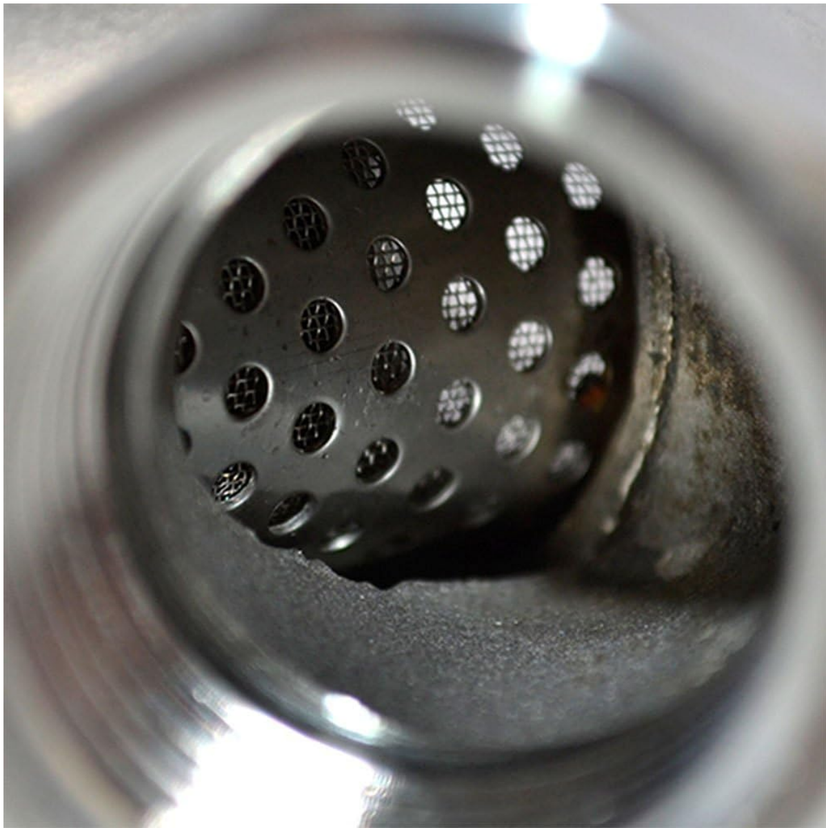
Figure 4: Internal view of the mesh filter screen, which collects particles.
