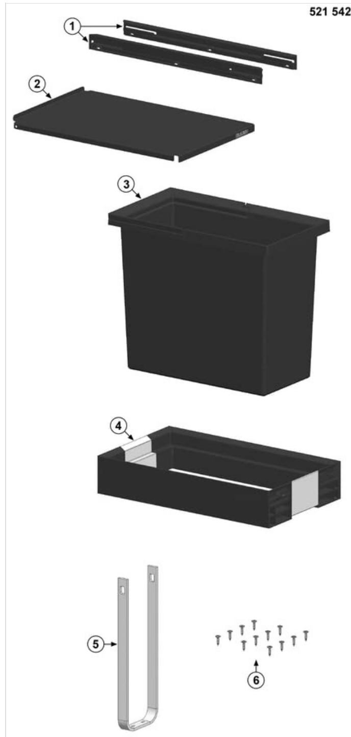
Image: Exploded view diagram showing individual parts of the BLANCO Flexon II system, including mounting rails (1), lid (2), waste container (3), frame (4), and mounting bracket (5) with screws (6).
