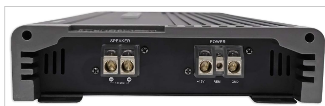
Image 4.1: Power and speaker output terminals of the Soundstream AR1.8000D amplifier.
