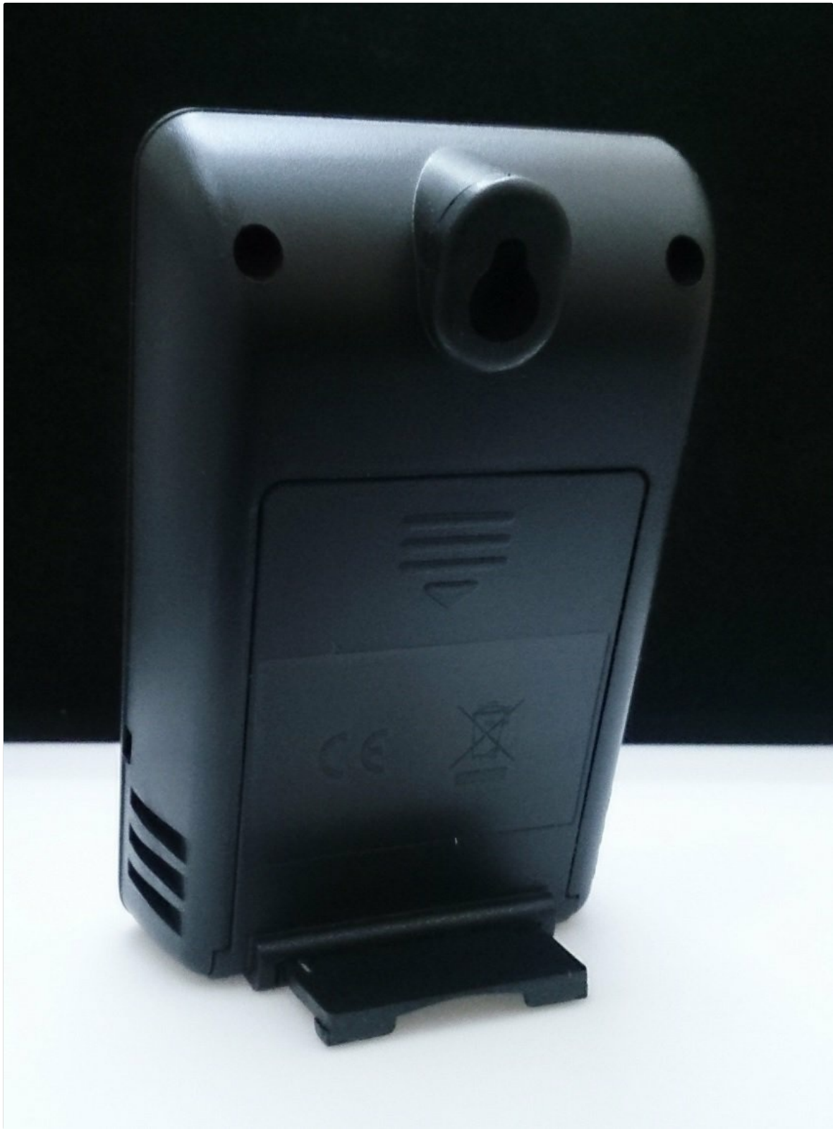
Figure 5: Rear view of the wireless remote sensor, indicating the battery compartment and mounting options.
