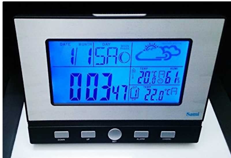
Figure 1: Front view of the Sami LD-1105N Wireless Weather Station main unit. The large LCD screen displays various weather data and time. Control buttons are located at the bottom edge.
