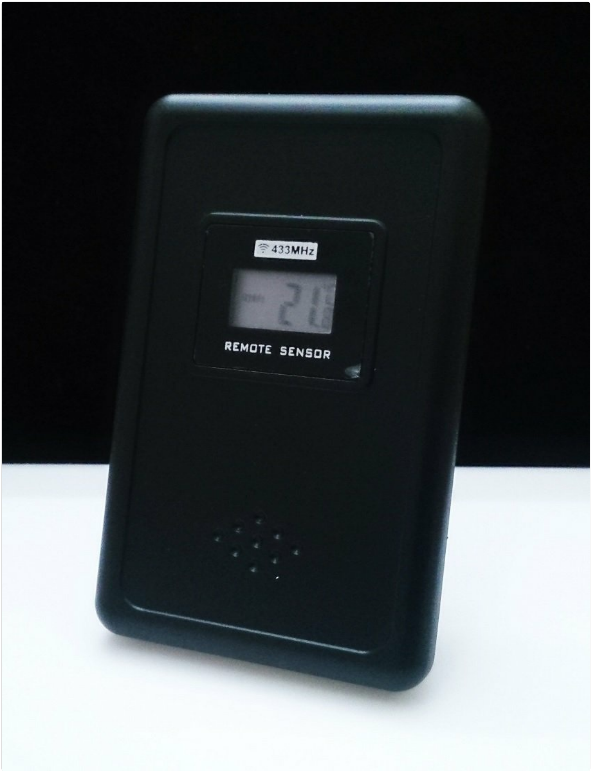
Figure 4: Front view of the wireless remote sensor. It has a small display showing its current channel and temperature.
