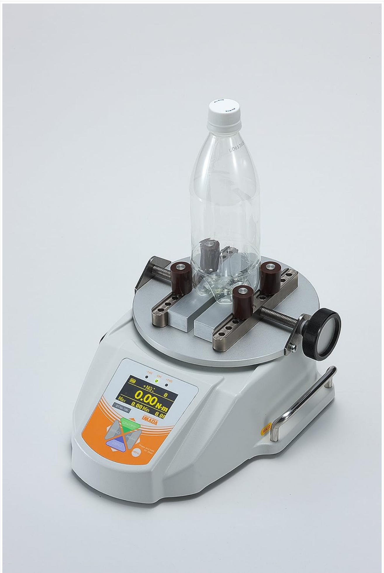
Figure 3.1: A sample bottle placed on the DTXA-10N's standard table, ready for testing.
