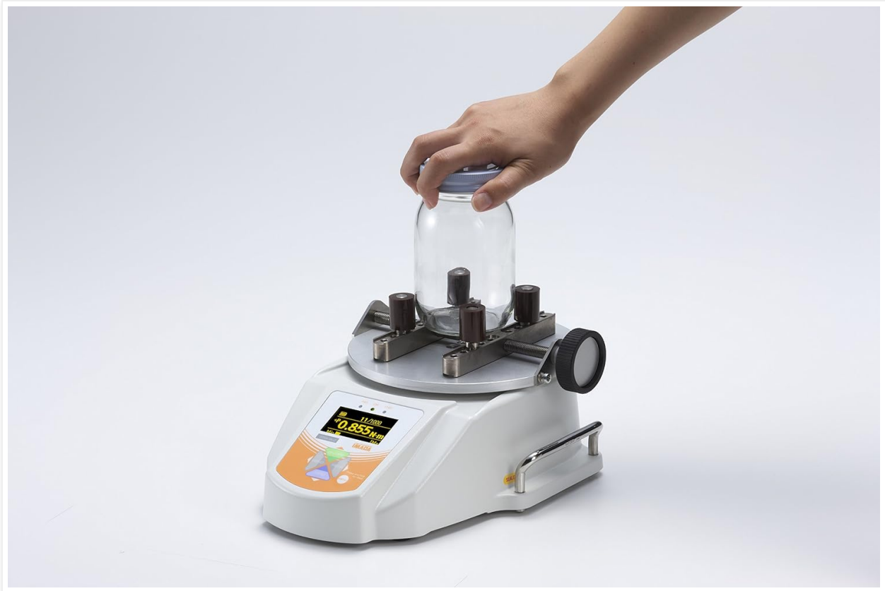
Figure 4.1: Proper placement of a sample jar on the tester's platform.
