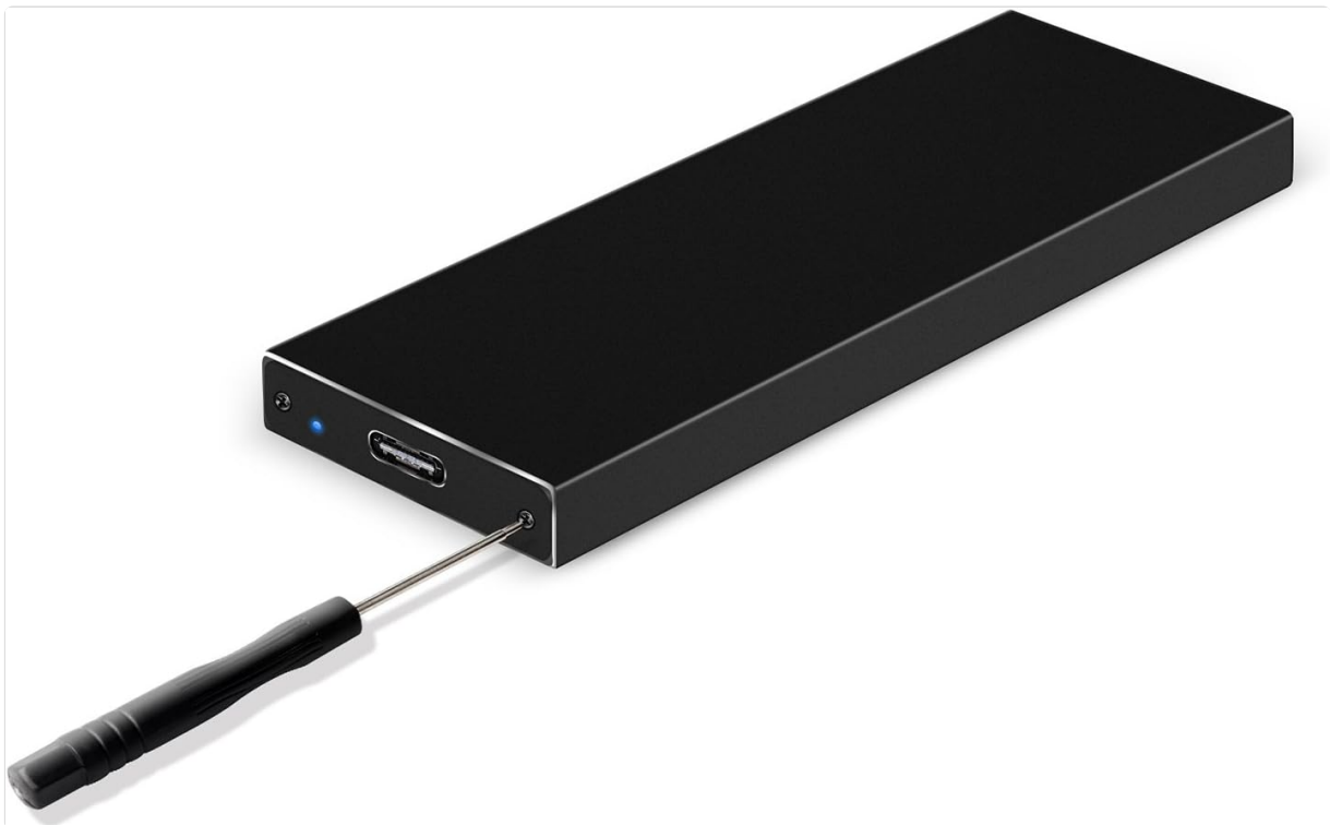
Figure 3.3: A screwdriver being used to secure the end cap of the MAIWO K16N enclosure, completing the assembly process after the SSD has been installed.
