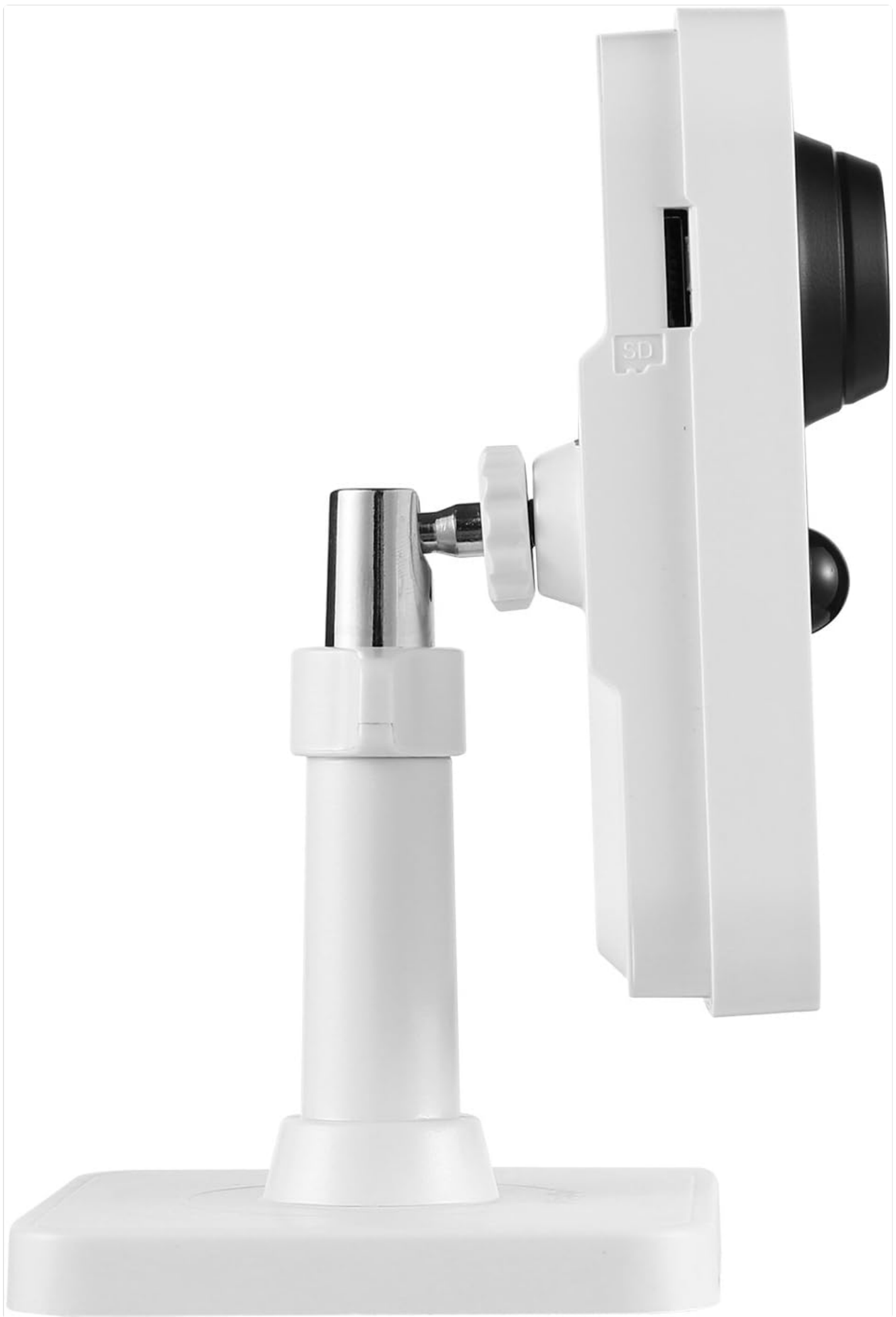
Image: The side of the ANNKE i61dr camera, showing the accessible SD card slot for local storage.
